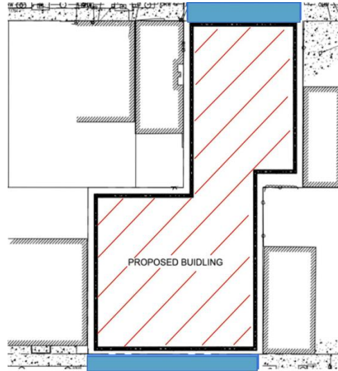
Figure 19. Shown in red hatching is the proposed roof area for the building, while the blue boxes indicate all areas where the two detention vaults could be placed.
