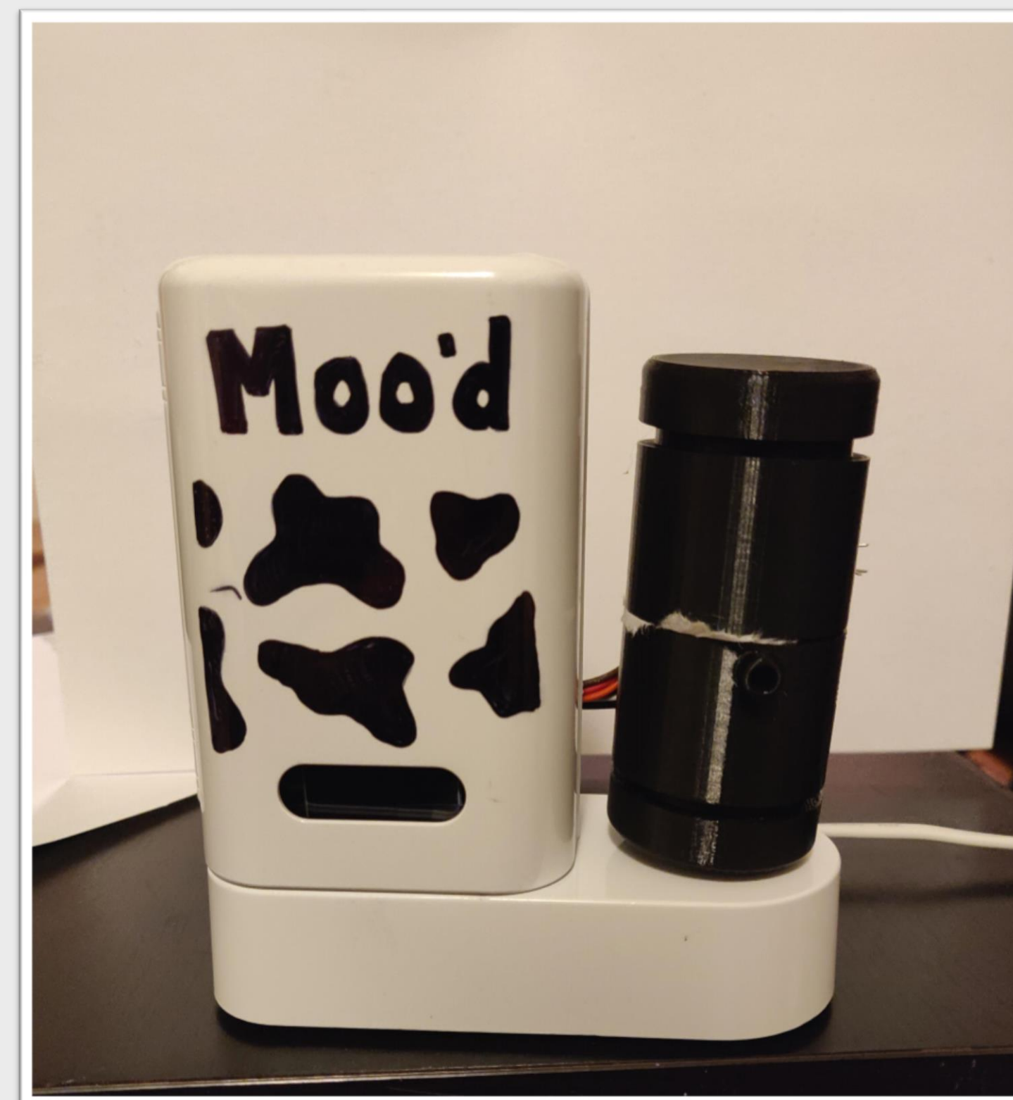
Figure 1: The Moo'D Casein Allergy Sensor. Main device housing to the left, casein separation canister to the right.
