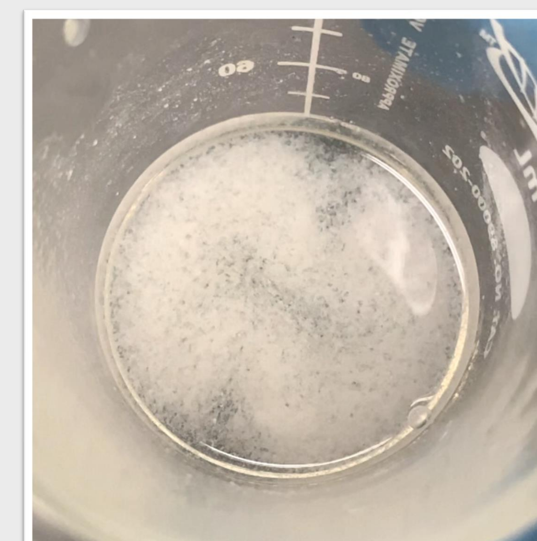
Figure 7: Precipitated casein after the addition of 4-5 drops of 10% acetic acid. The casein is now visible and can be filtered out.
