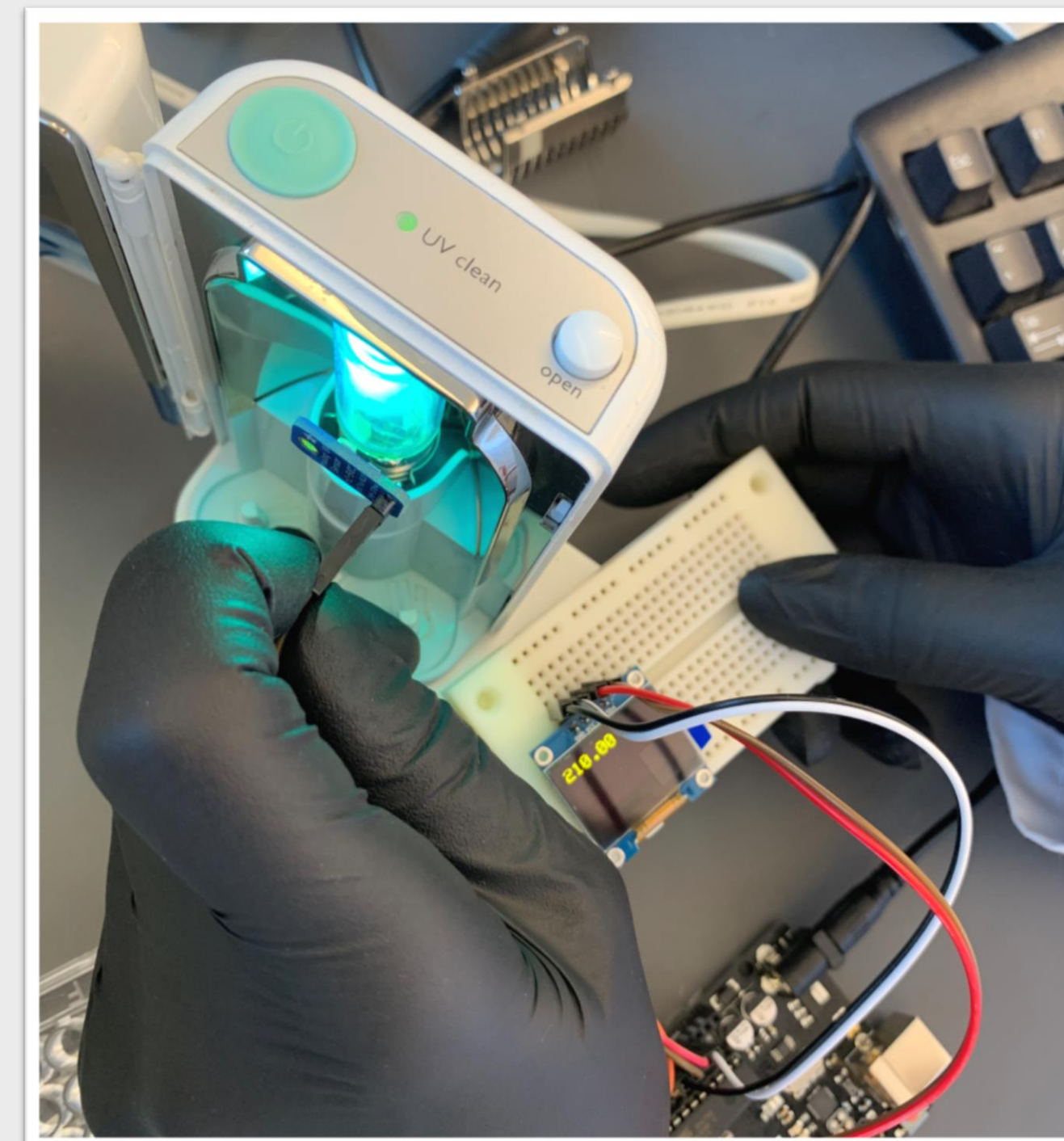
Figure 2: Inside of the device showing the UV light source and UV sensor testing. Holding the sensor almost directly on the light output an analog value of 218.
