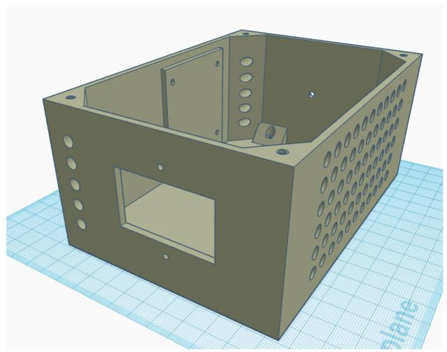
Figure 30: Smart Hub Enclosure <u>https://drive.google.com/file/d/1d3GbehmJC5RpVB5hYlpk8KMhre2BrHHy/view?usp=share\_link</u>
