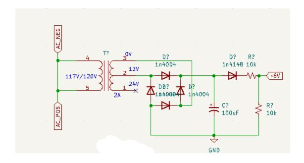
Figure 26: Rectifier Circuit Schematic
