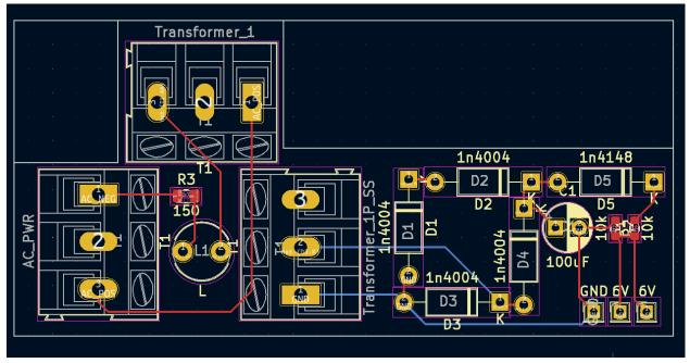
Figure 27: Smart Plug PCB Design
