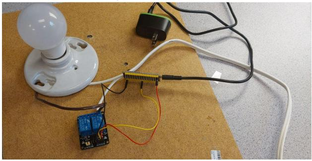
Figure 14: Smart Plug Circuit
