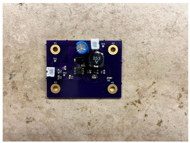
Figure 17: Fully assembled Buck Converter
