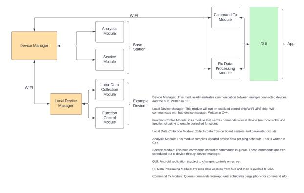
Figure 29: High Level Software
