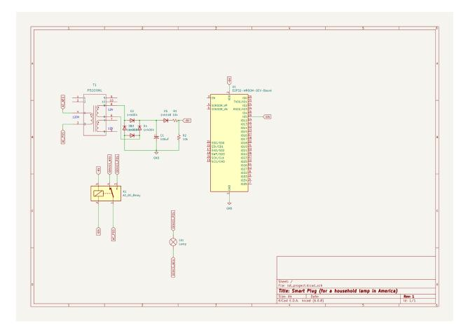
Figure 12: Smart Plug Hardware schematic
