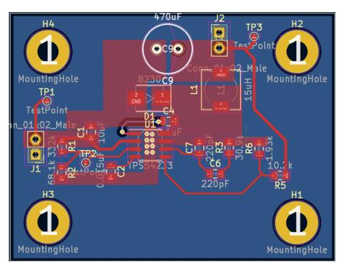
Figure 16: Buck Converter PCB
