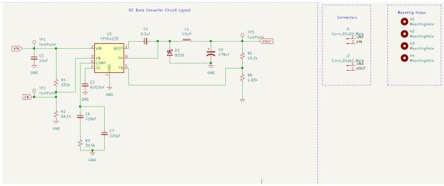
Figure 15: Buck Converter Schematic.
