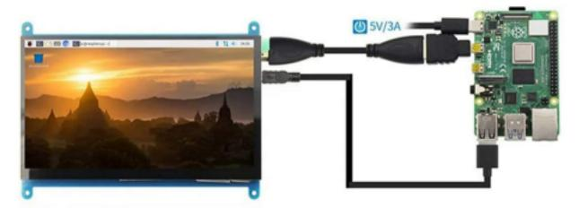
Fig. 4.6.2.2: Capacitive Touch Screen Connections to Raspberry Pi
