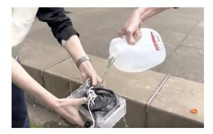
Figure 5.2.7.5: Weather Resistance Test
