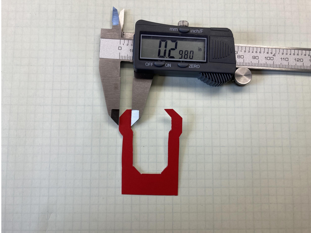
Figure 5.6.3.5: Demonstrating that the width of the cardstock template is larger than minimum required tolerance between bracket and the connector, proving that the template can be used to visually verify the clearance requirement.
