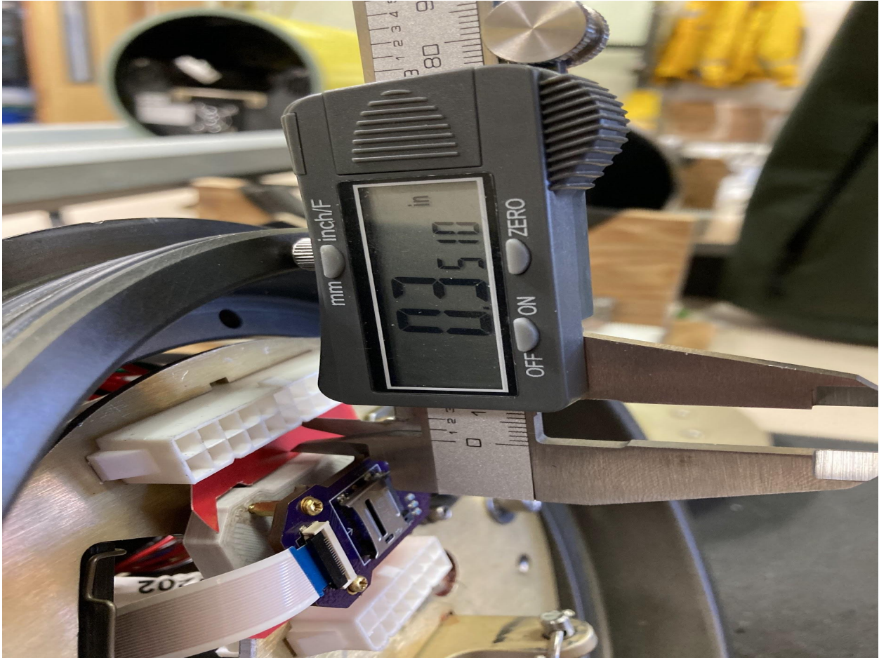
Figure 5.6.3.3: Demonstrating that the clearance requirement between the top white snap connector and the 3D printed bracket is greater than the required minimum of 0.25 inches.
