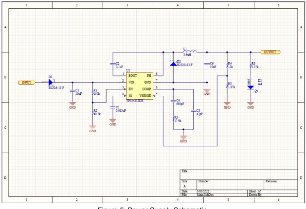
Figure 5: Power Supply Schematic
