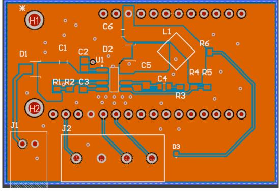
Figure 11: Top layer of PCB layout
