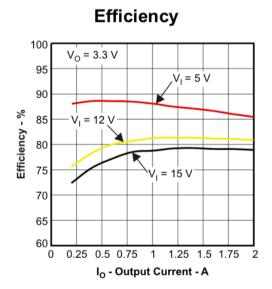
Figure 30: TPS4232 efficiency graph
