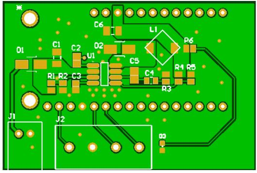
Figure 13: Top view of Gerber file generated PCB
