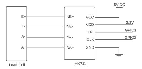
Figure 8: Schematic of force sensor block.
