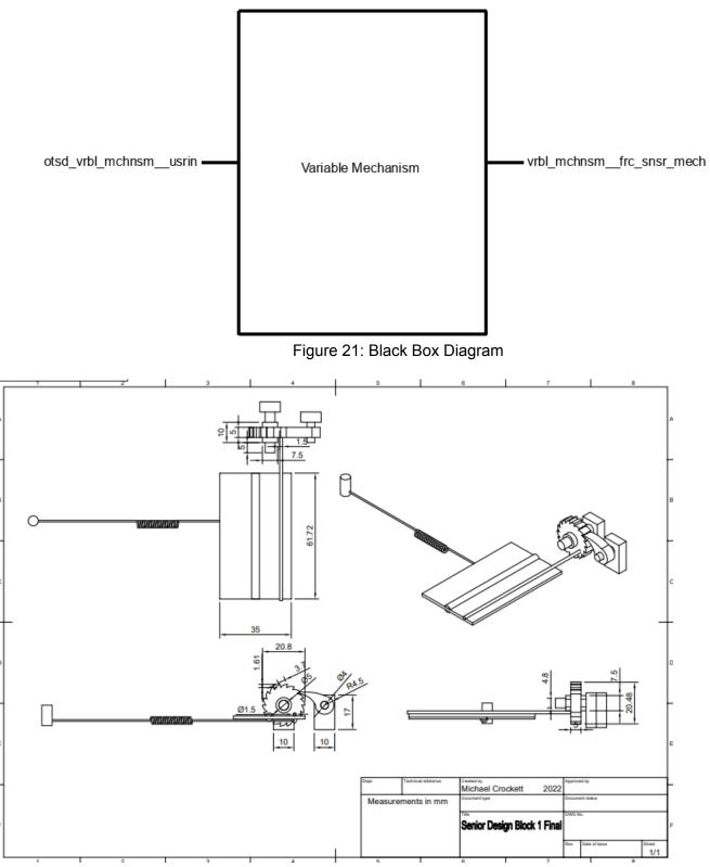
Figure 22: Mechanism Drawing
