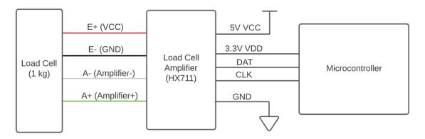
Figure 7: Wiring diagram of the force sensor block.
