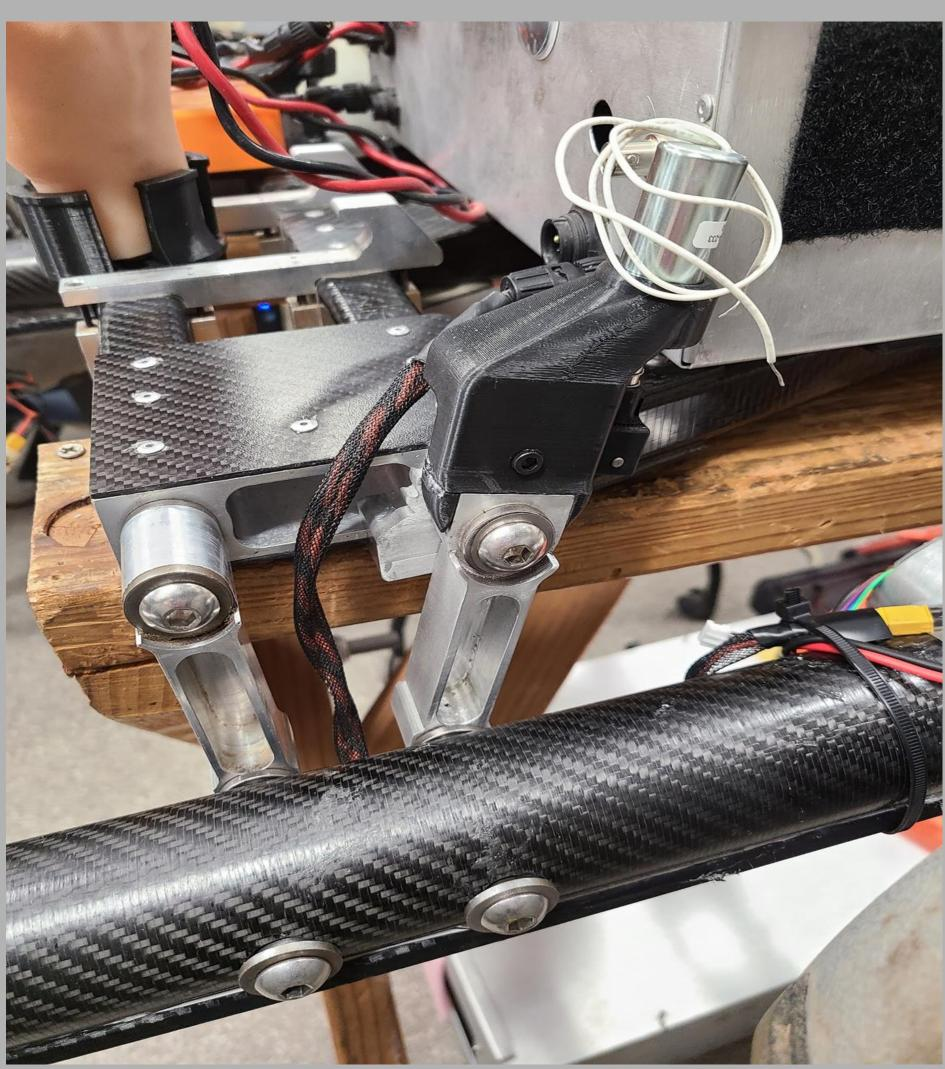
The locking mechanism is comprised mostly of water jet and machined aluminum with a 3D printed PLA solenoid bracket.
