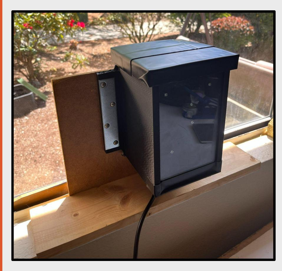
The purpose of this device is to prevent bird-window collisions. When the device detects a bird flying towards a window, the device will alert the bird to allow it to change its flight path away. To accomplish this, the design utilizes two main sections, a sensors/detection section and a deterrents section.
