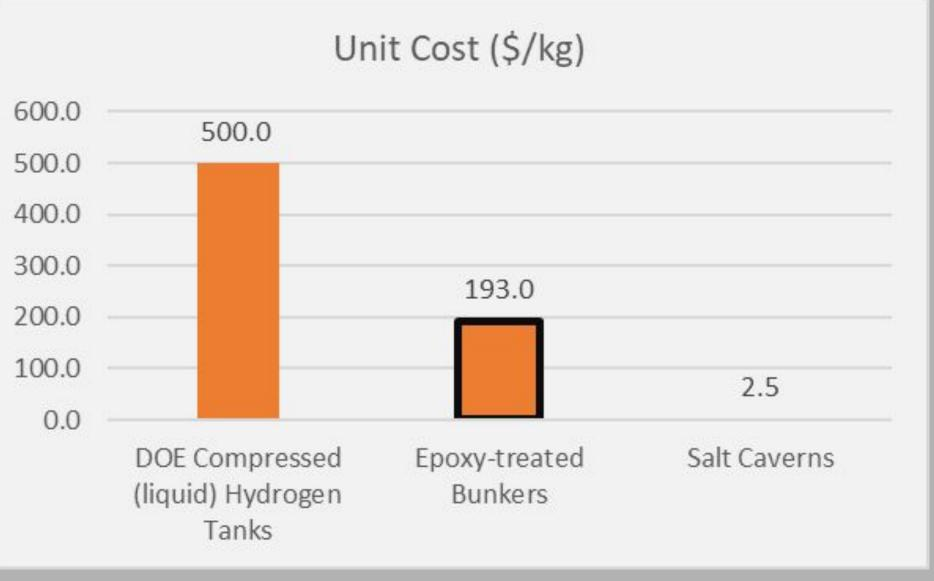
This epoxy resin treatment is a competitive option compared to other storage methods due to its lower cost and high versatility.
