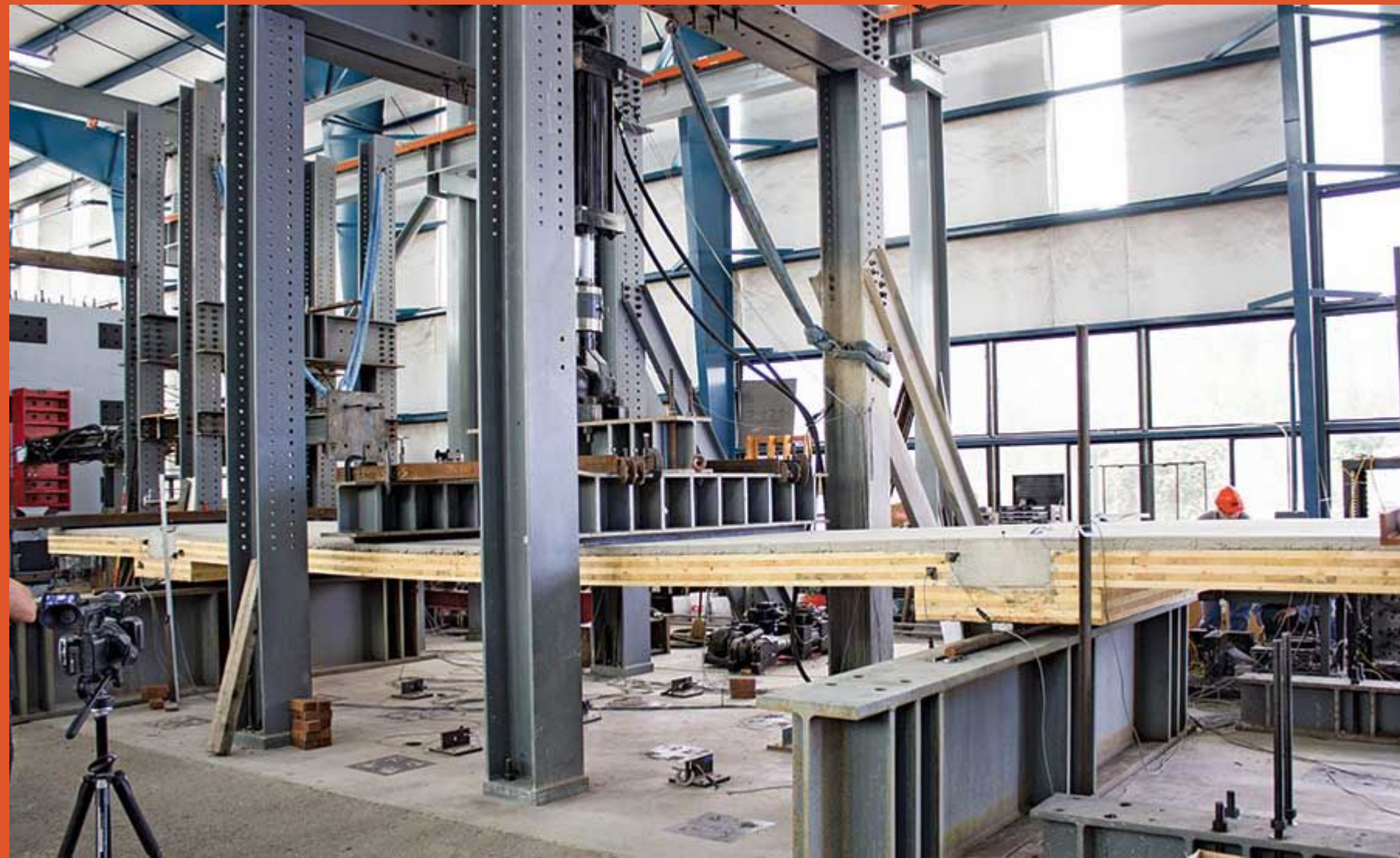
Fig 1: The hydraulic test rig that is used to test the structural materials
