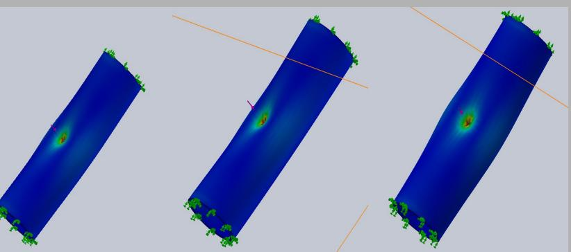
Simulating stress tests on SolidWorks of cylinders composed of different biodegradable plastics
