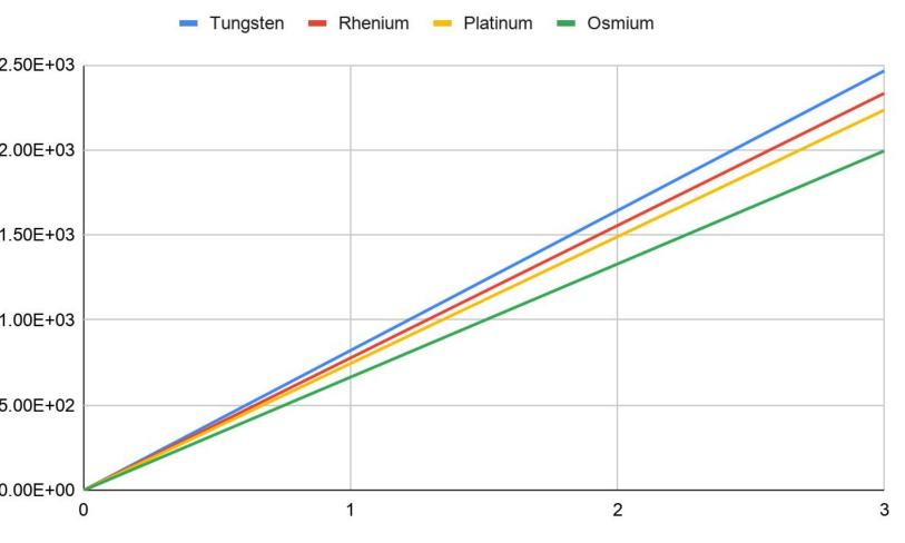
Modeling the amount of heat needed to bring different filaments up to cauterizing temperatures of 1700-2200'K. • Tungsten, aluminum, copper, tin & aluminum bronze
