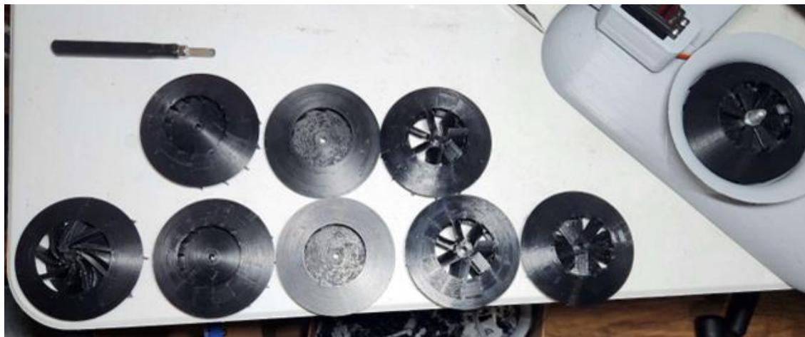
Figure 4: Five of the six fan iterations (4 pairs seen above) produced during the first vehicle iteration.
