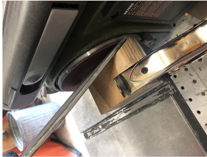
Fig. 31 Fin Bevel Jig for the Finalized Fins
