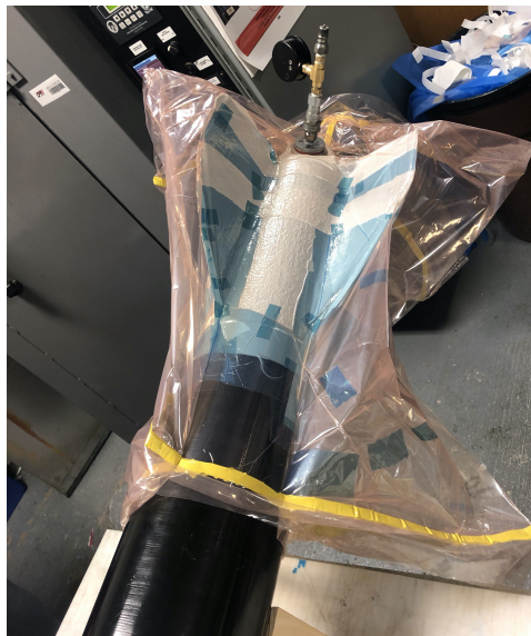
Fig. 34 Bagged Tip-to-Tip Layup
