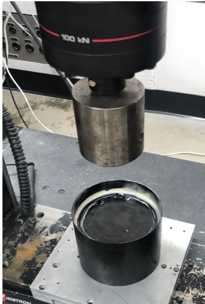
Fig. 25 Testing of Bulkhead w/ Coupler
