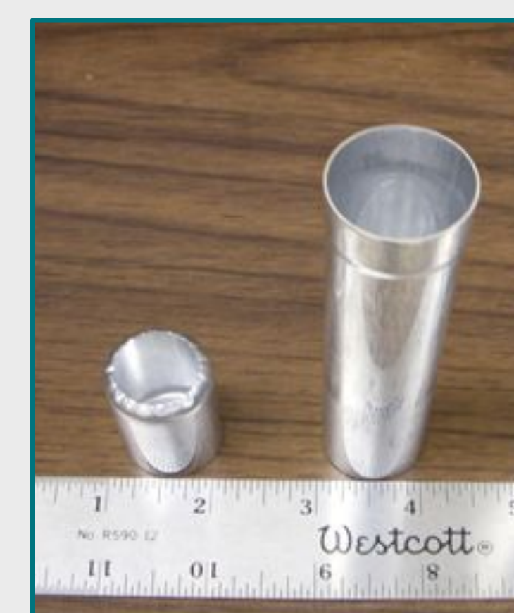
Left: TRIGA Core Map, ICIT facility (F12) Right: Top: Example of irradiation vial with small inner quartz ampoule Bottom: Example OSTR outer aluminum irradiation tube with the top and bottom separated
