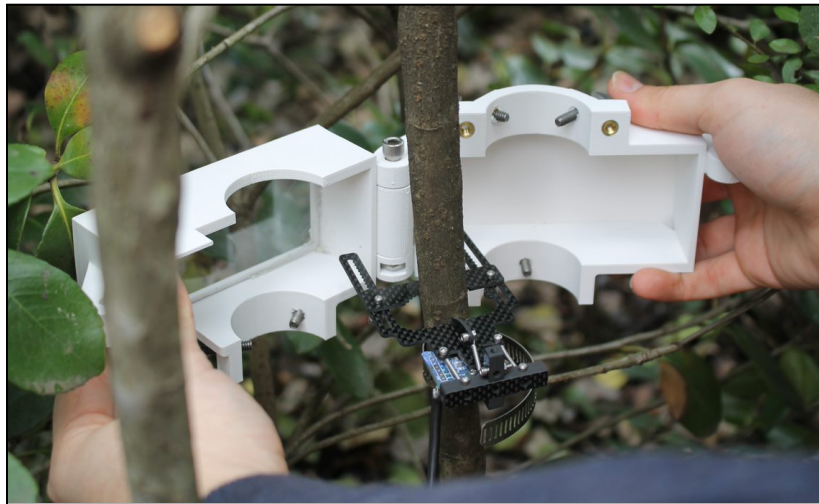
Figure 15. Installing protective case around the V2.3 dendrometer carbon fiber prototype.
