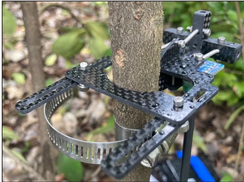
Figure 13. V2.3 prototype recording diameter changes on a plant outside the OPEnS Lab.
