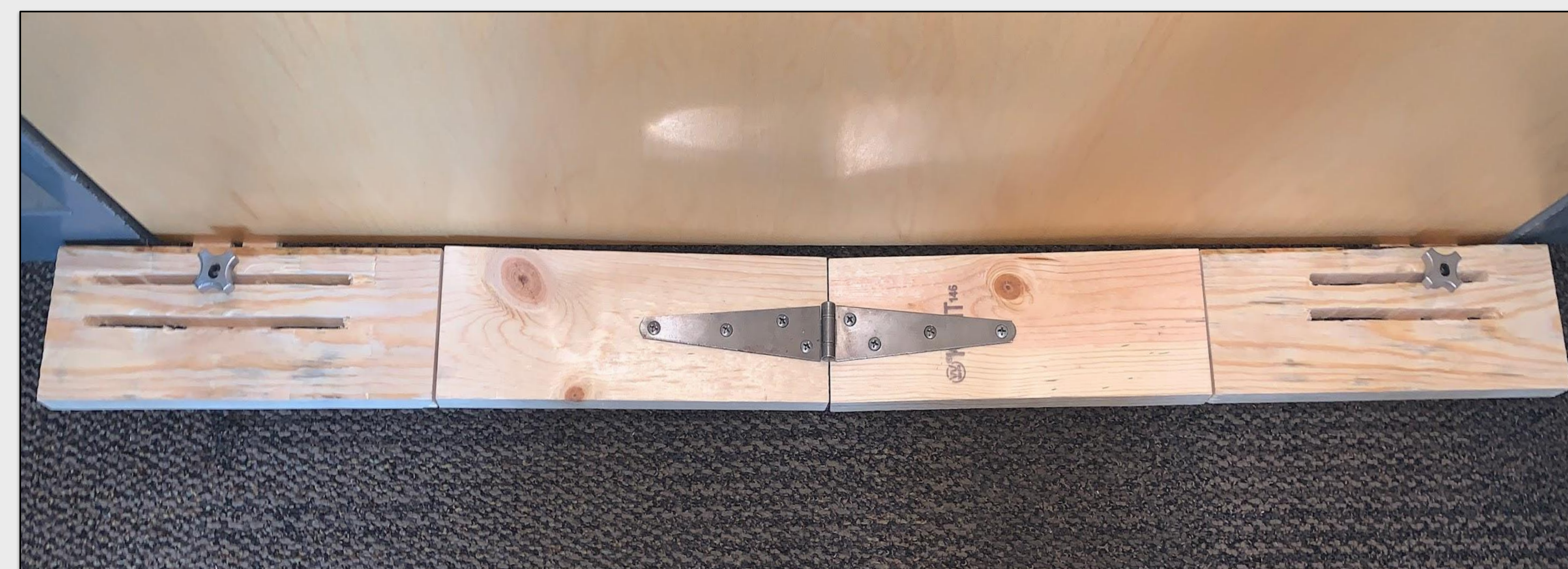
Figure 2: The door stop is shown deployed on the secure side. The Z-Axis locking pins are not shown to be in use.
