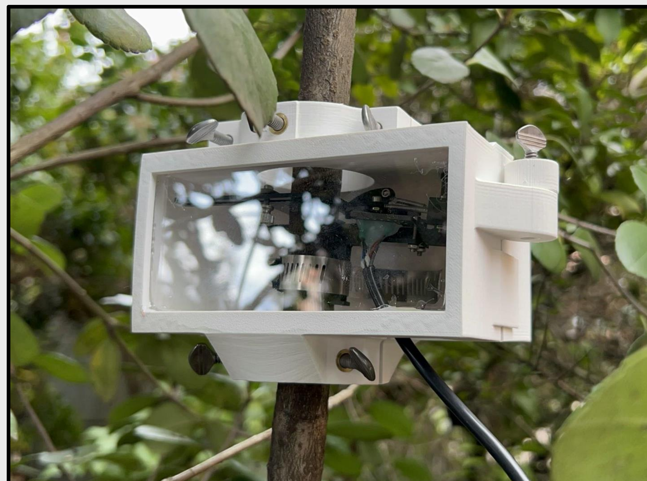
Installed dendrometer with protective casing
