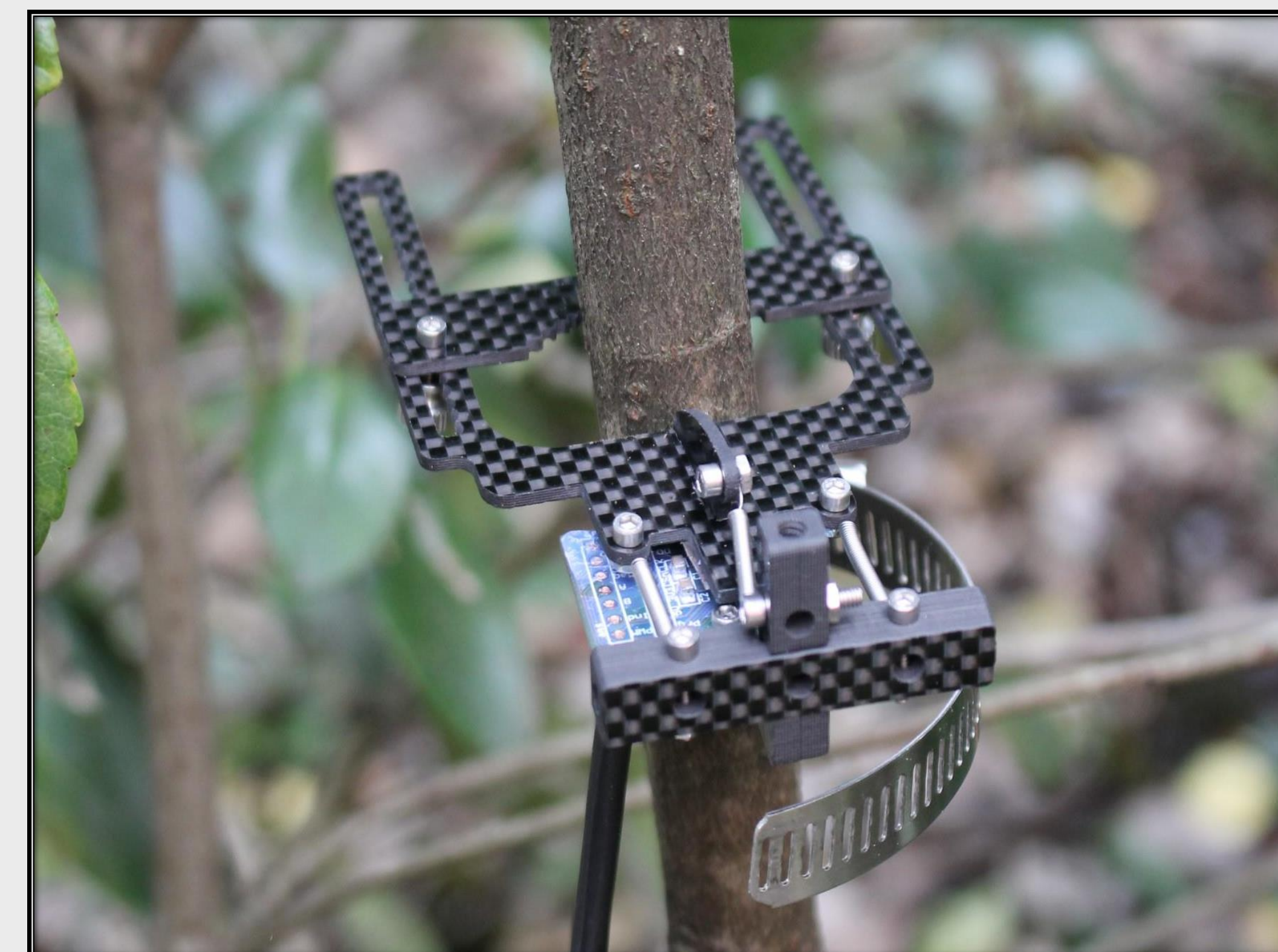
The Dendrometer: Installed onto stems to measure stem diameter fluctuations
