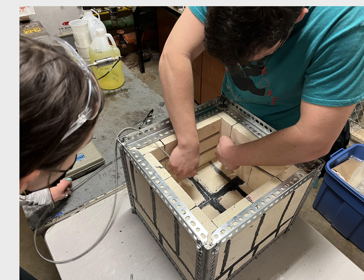
Pinning heating coil into routed channels
