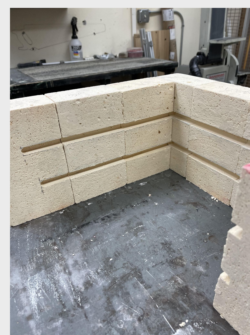
Channels in kiln brick for heating coil made on router table
