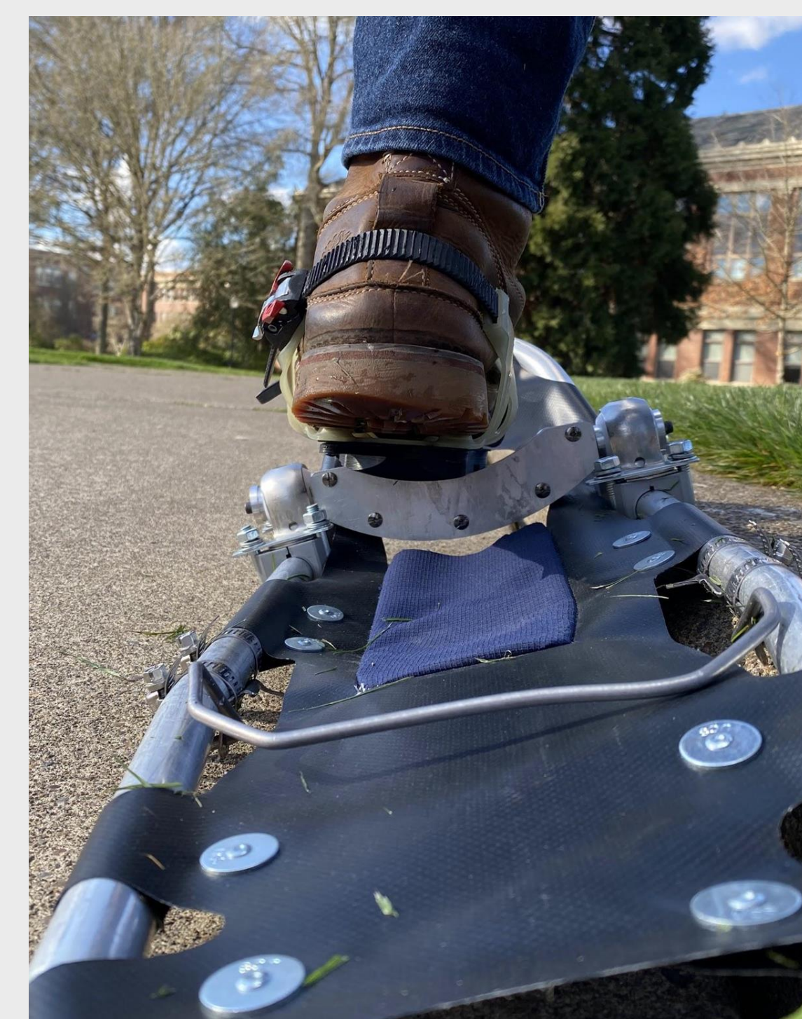
Roll articulation for sidehill climbing
