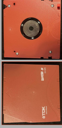
Figure 5: LTO Cartridge. Right side shows the top, the left side shows the locations of the screws that are punched out.
