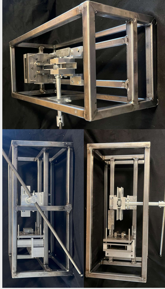
Figure 1: Full build of LTO Cartridge Punching Mechanism seen from three views.
