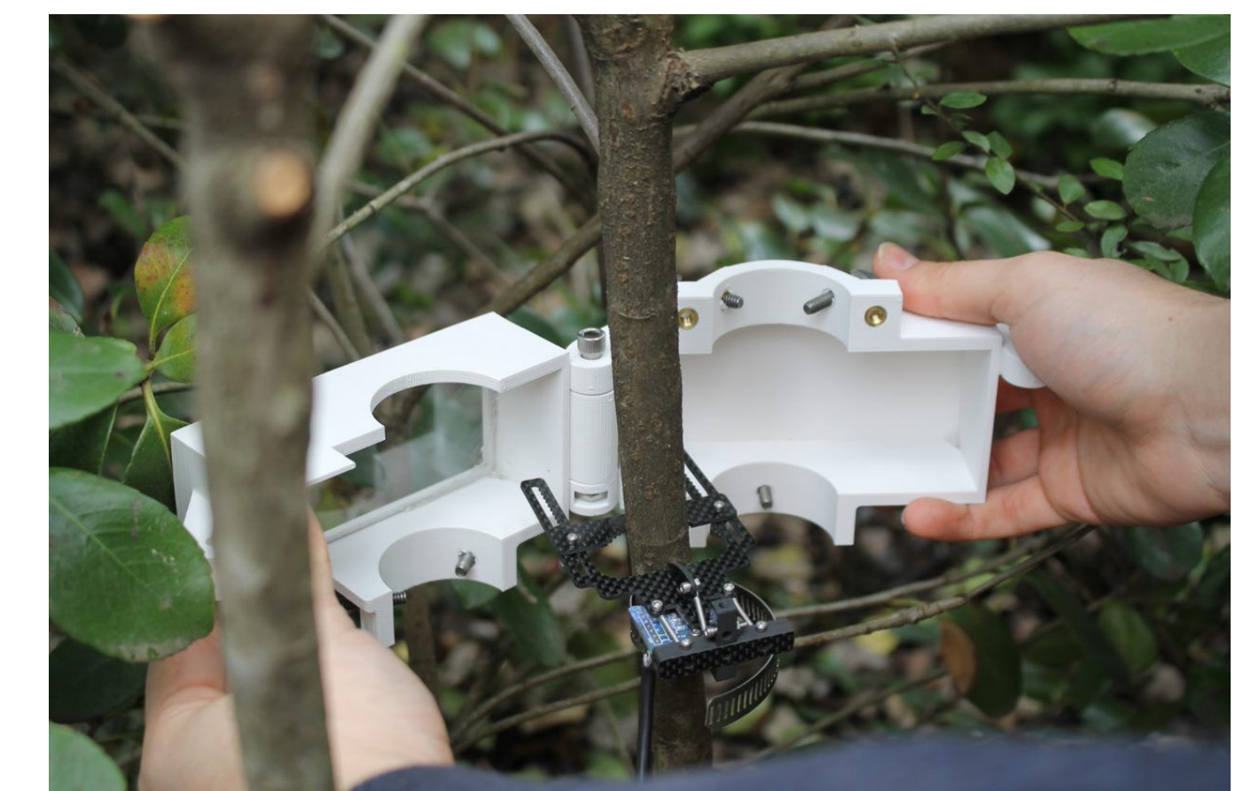
Figure 11: Carbon fiber V2 dendrometer installed on a plant outside the OPeNS Lab. This was used to test the reliability of the new V2 design with data collection as well as the robustness of the 3D printed protective enclosure
