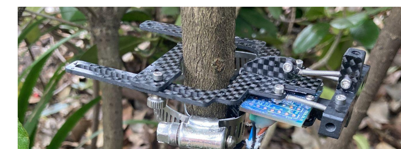
Figure 10: 3D printed dendrometer installed on a blueberry plant at Lewis-Brown (LB) Farm in Corvallis, OR. The initial rounds of prototype testing were conducted with 3D printed parts of the new dendrometer and changes validated.
