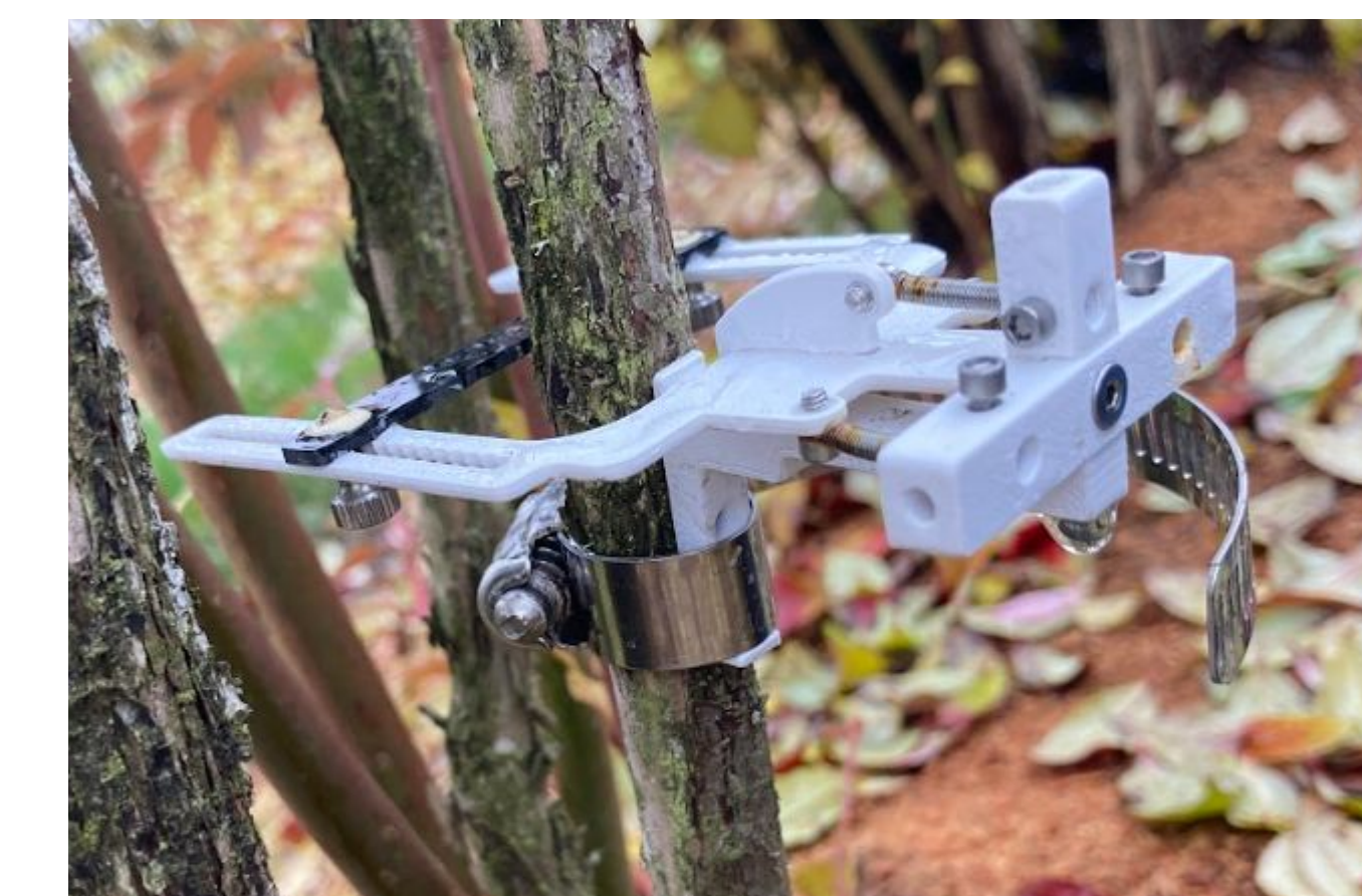
Figure 10: 3D printed dendrometer installed on a blueberry plant at Lewis-Brown (LB) Farm in Corvallis, OR. The initial rounds of prototype testing were conducted with 3D printed parts of the new dendrometer and changes validated.
