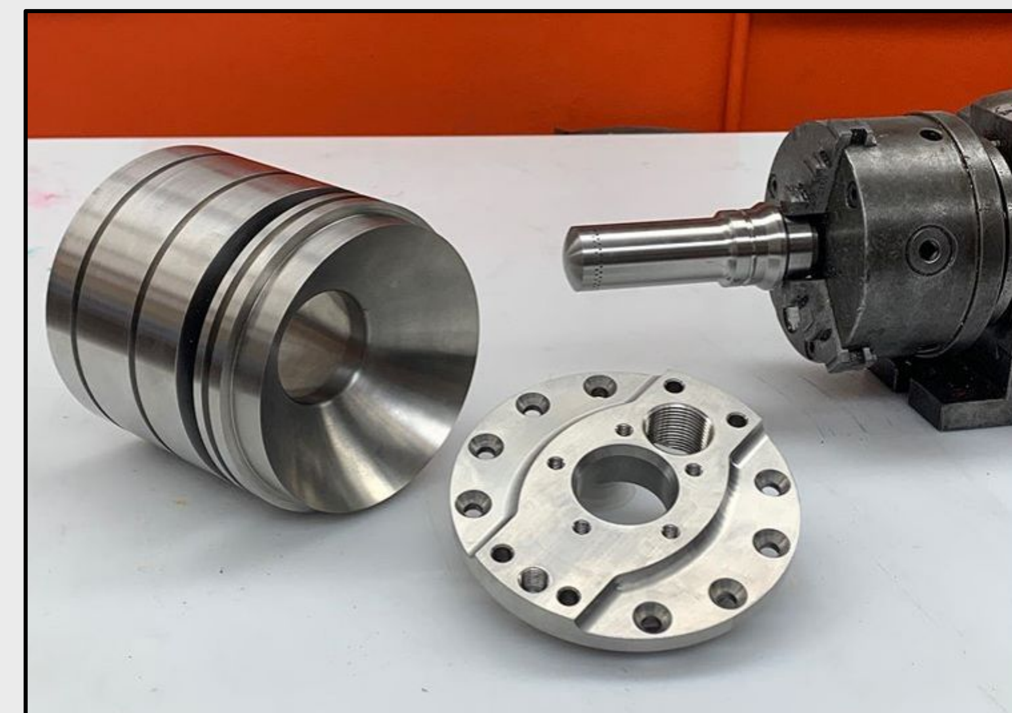
Left to right: test nozzle, injector plate, pintle
