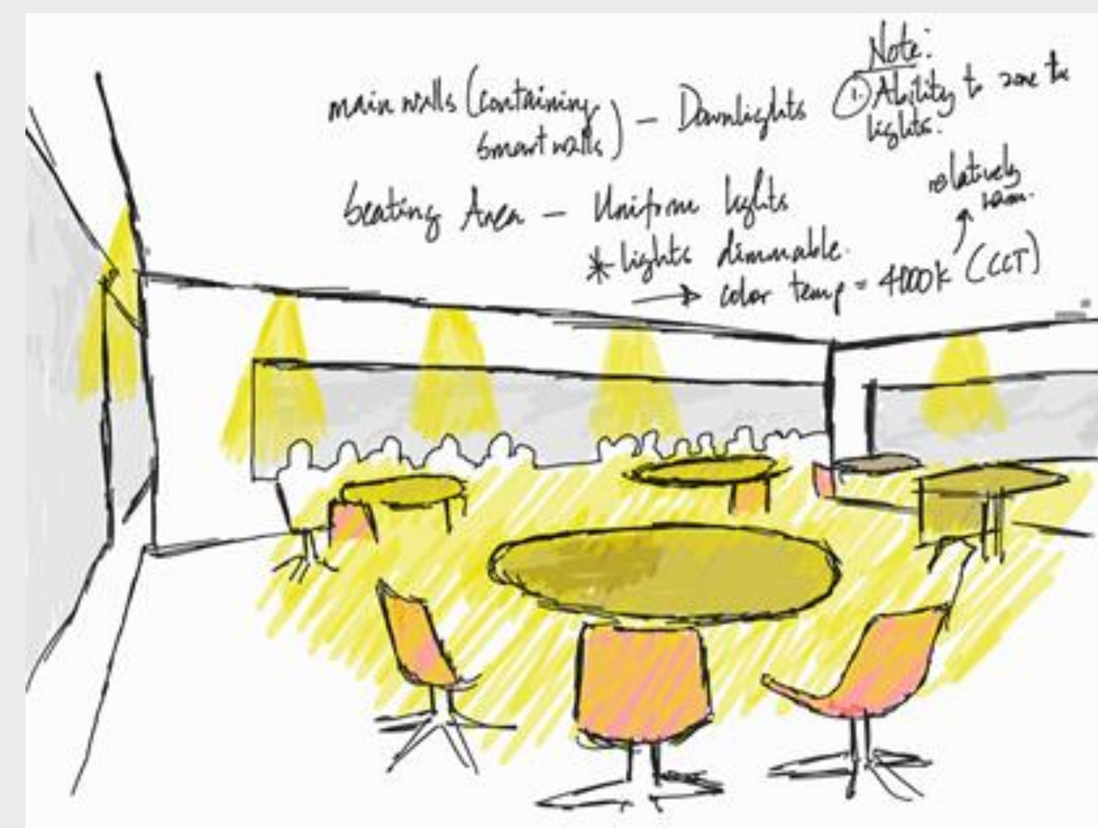
SCHEMATIC SHOWING LIGHT DISTRIBUTION IN THE LEARNING STUDIO CLASSROOM
