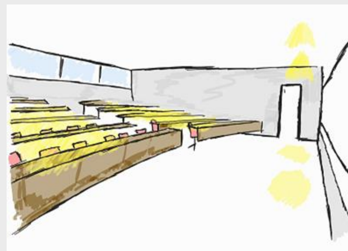
SCHEMATIC SHOWING LIGHT DISTRIBUTION IN THE TIERED CLASSROOM
