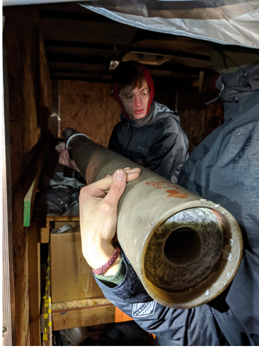
Figure 6: Propellant grains glued into thermal liner
