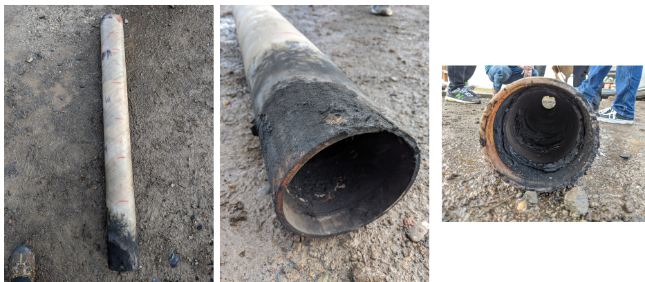
Figure 32: Damage to thermal liner
