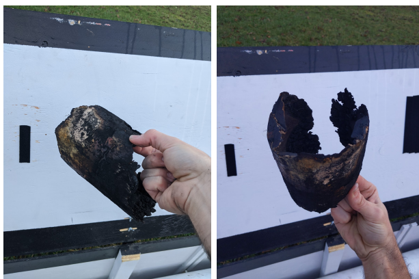
Figure 33: Damage to casting tube
