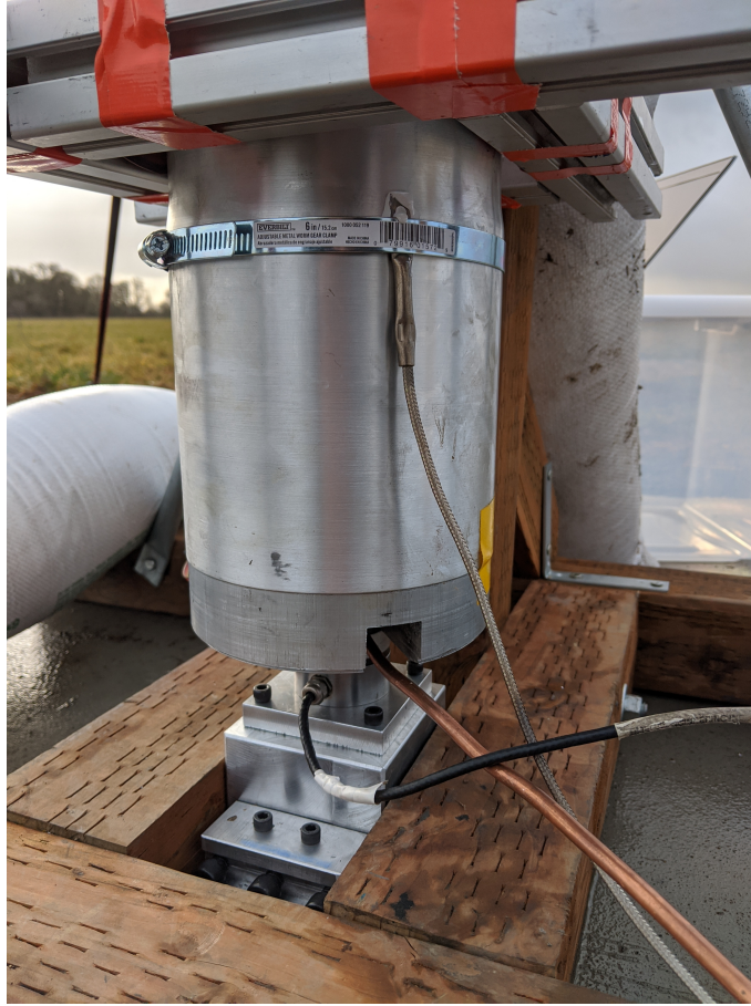
Figure 18: Load-cell and pressure transducer setup
