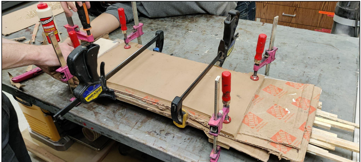
Figure 3. First attempt at gluing the board using wood to compress the fronds into a plane.
