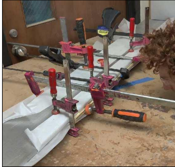
Figure 4. Revised method for gluing the second board using aluminum plate to create a flatter final board.
