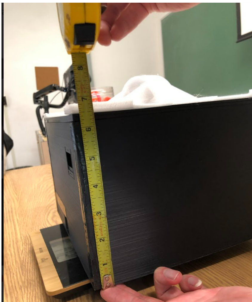
Figure 38: Laser Painter system height (7.5 inches to handle)
