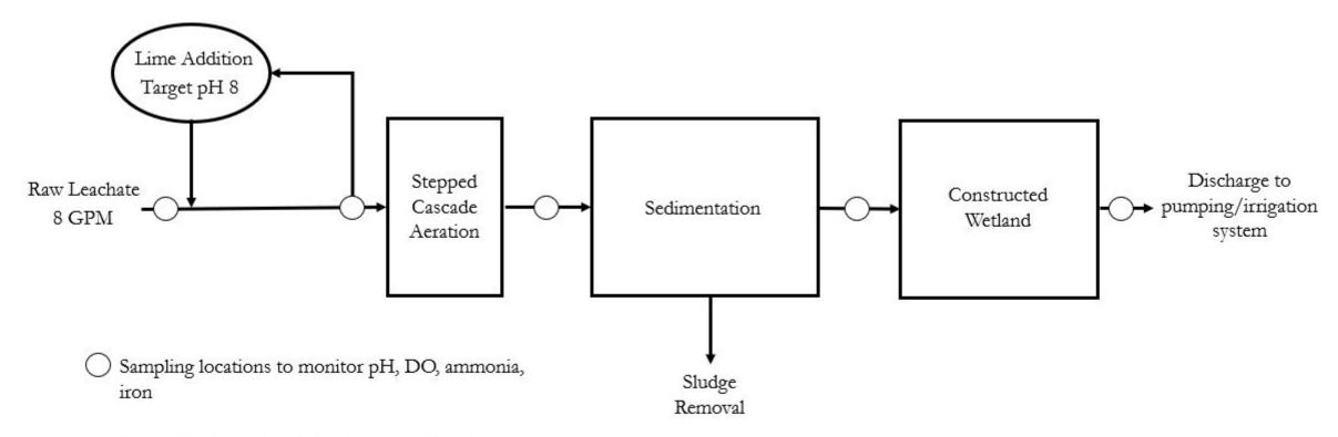
Lime addition system includes recycle loop to ensure pH target is met.
