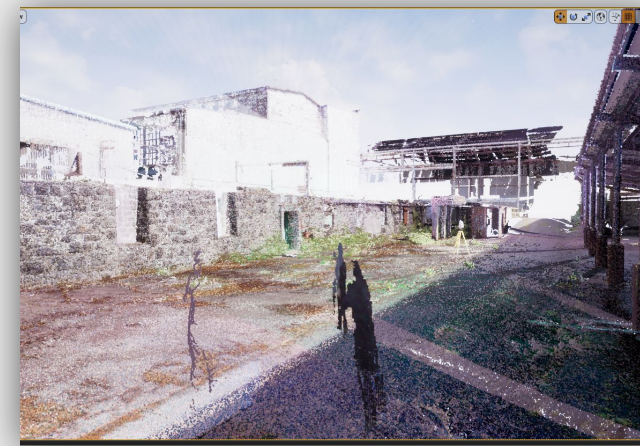
Fig 3. View of LiDAR scan data brought directly into Unreal Engine
