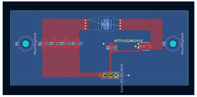
Figure 5.5: Strobe Light PCB Layout
