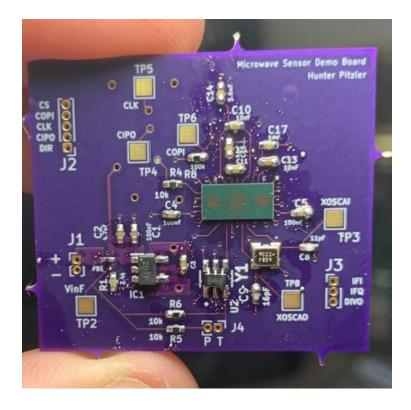
Figure 4.6: Microwave Sensor PCB Front Side
