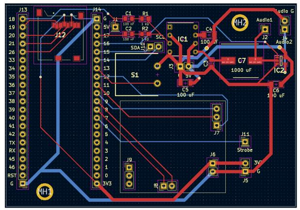
Figure 6.1: Control Board PCB Layout
