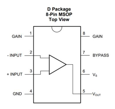
Figure 4.14: OpAmp Pin Configuration and Functions
