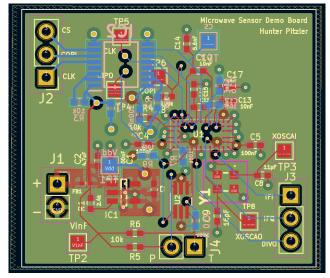
Figure 5.2: Microwave Motion Detector PCB Layout
