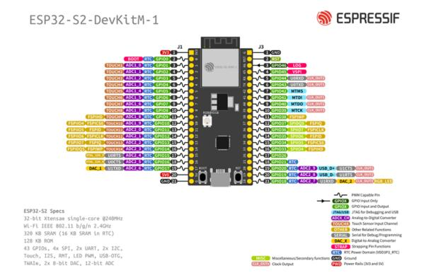
Figure 4.27: ESP32-S2 DevKitM-1 Pin Layout
