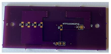
Figure 6.14: Strobe Light Board Front Unpopulated PCB
