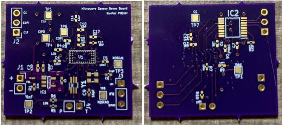
Figure 6.6: Unpopulated Motion Sensor PCB (Front and Back)
