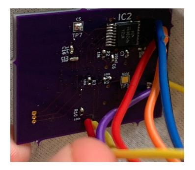
Figure 4.7: Microwave Sensor PCB Back Side
