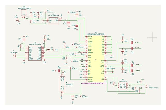
Figure 4.5: Microwave Sensor Schematic
