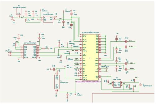
Figure 6.4: Motion Sensor Schematic
