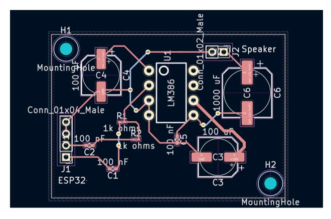
Figure 4.17: Audio Amplifier PCB Design
