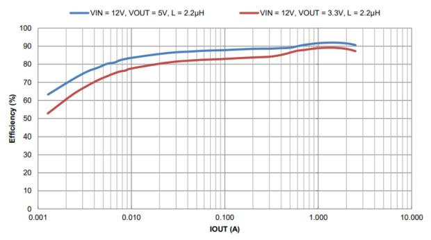
Figure 2. Efficiency vs. Output Current
