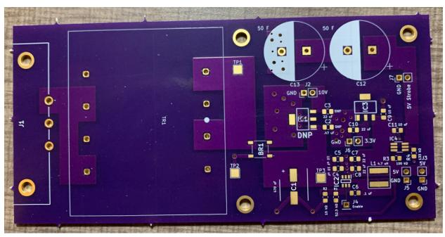
Figure 6.9: Power Supply Board Unpopulated PCB
