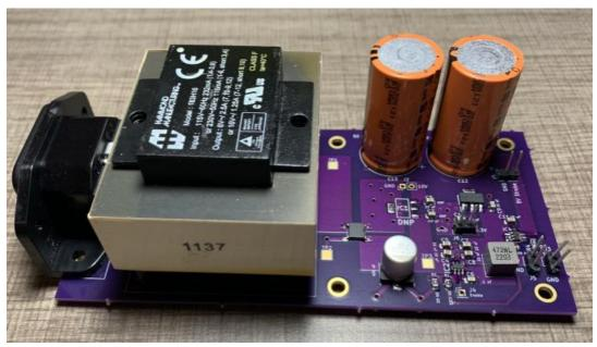
Figure 6.10: Power Supply Board Populated PCB
