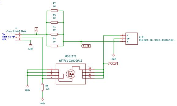
Figure 6.12: Strobe Light Schematic Design
