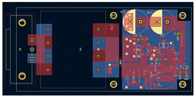
Figure 6.7 Power Supply Board PCB Layout
