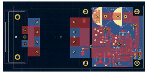
Figure 5.3: Power Supply PCB Layout
