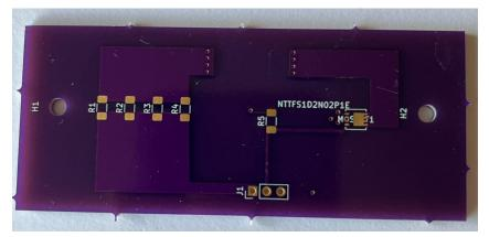
Figure 4.24: Strobe Light Board Front Unpopulated PCB
