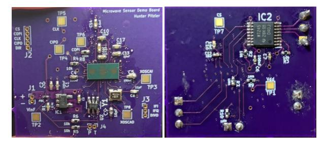
Figure 6.6: Populated Motion Sensor PCB (Front and Back)
