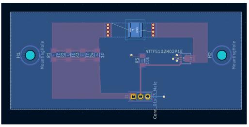
Figure 4.23: Strobe Light Board Back PCB Layout
