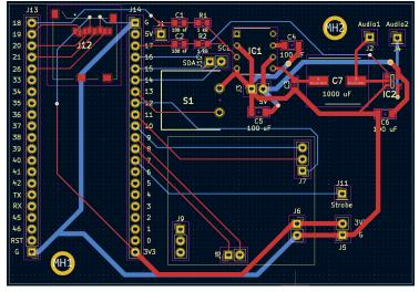
Figure 5.4: System Control PCB Layout
