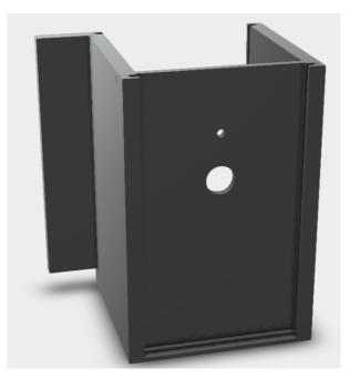
Figure 4.31: Front view of the enclosure's main body.
