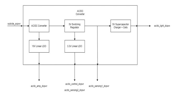
Figure 4.2: AC/DC Converter Internal Block Diagram
