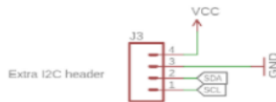
Figure 26: SIM7000-LTE-Shield Headers and Pinouts
