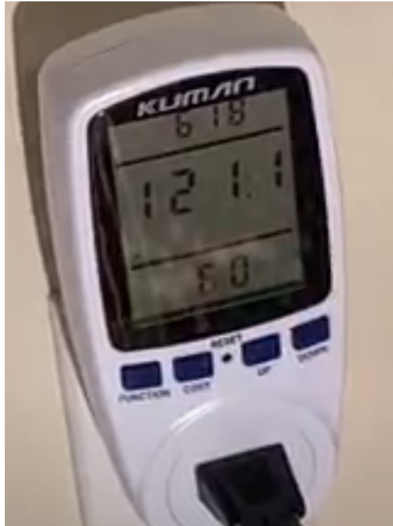
Figure 52: Meter showing voltage and frequency within 5% error
