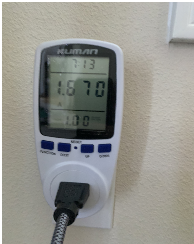
Figure 51: Meter showing current within 5% error
