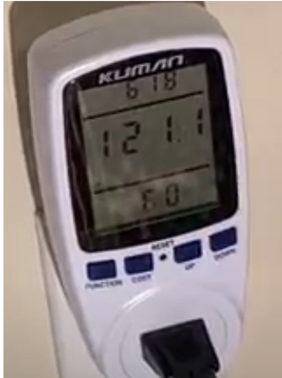
Figure 57: Meter showing voltage and frequency within 5% error
