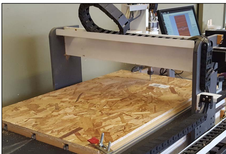
Cutting out ribs using CNC machine
