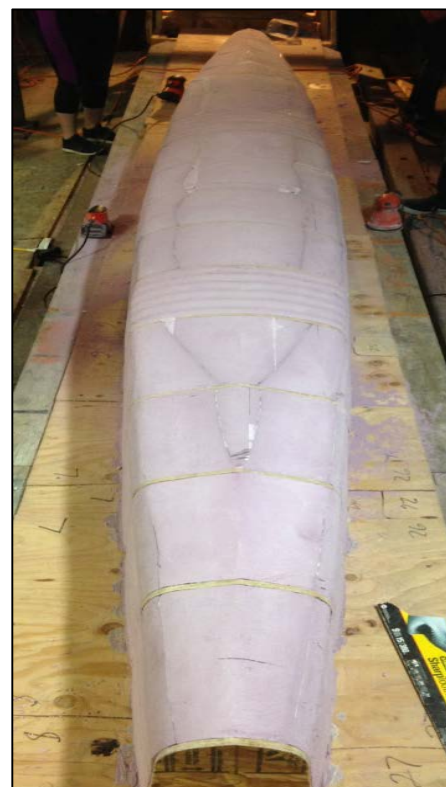
Shaping Foam to Ribs
