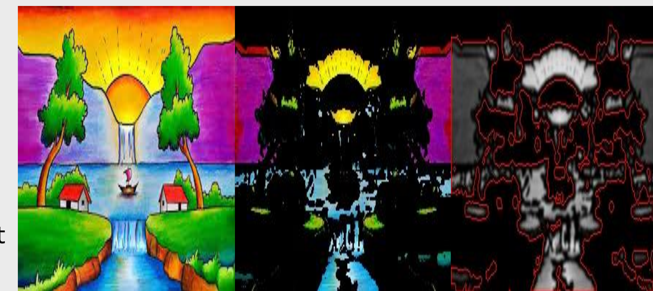
Fig 3. Masking and finding contours within image. Image 1 is loaded as RGB image and converted to HSV. It is masked for RGB duplex overlap to produce image, then converted to grayscale and blurred to prep it for finding its contours. Then the contours are analyzed against parameters to produce a risk score for each page based on coverage
