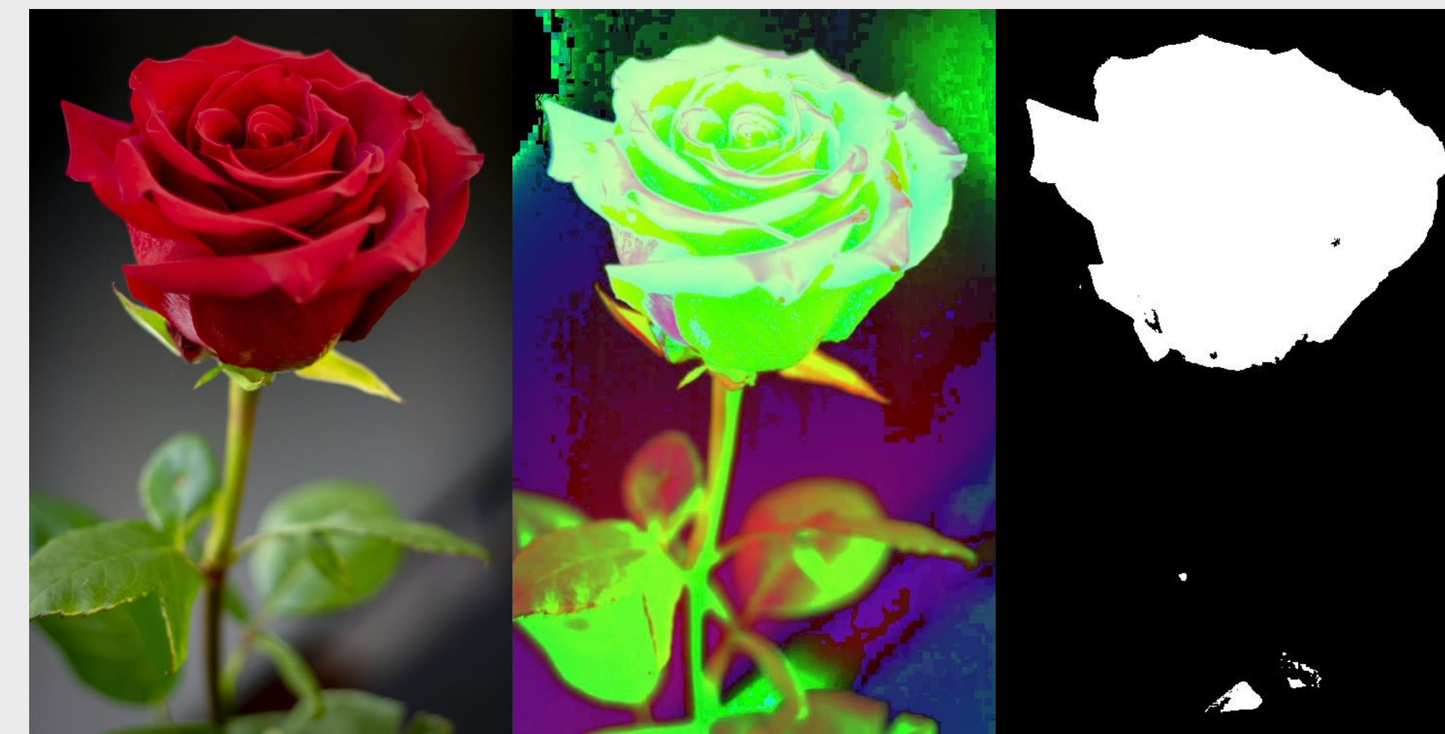
Fig 2. Three different operations done to an image in the wrinkle/curl algorithm. The image is loaded as an RGB image, converted to HSV, and then thresholding is applied to the pixels in the image that allows the algorithm to selectively pick pixels within the red hue area, which is shown in the rightmost picture
