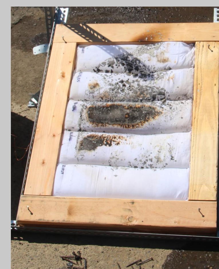
Figure 4: The SAP blanket roof after test completion
