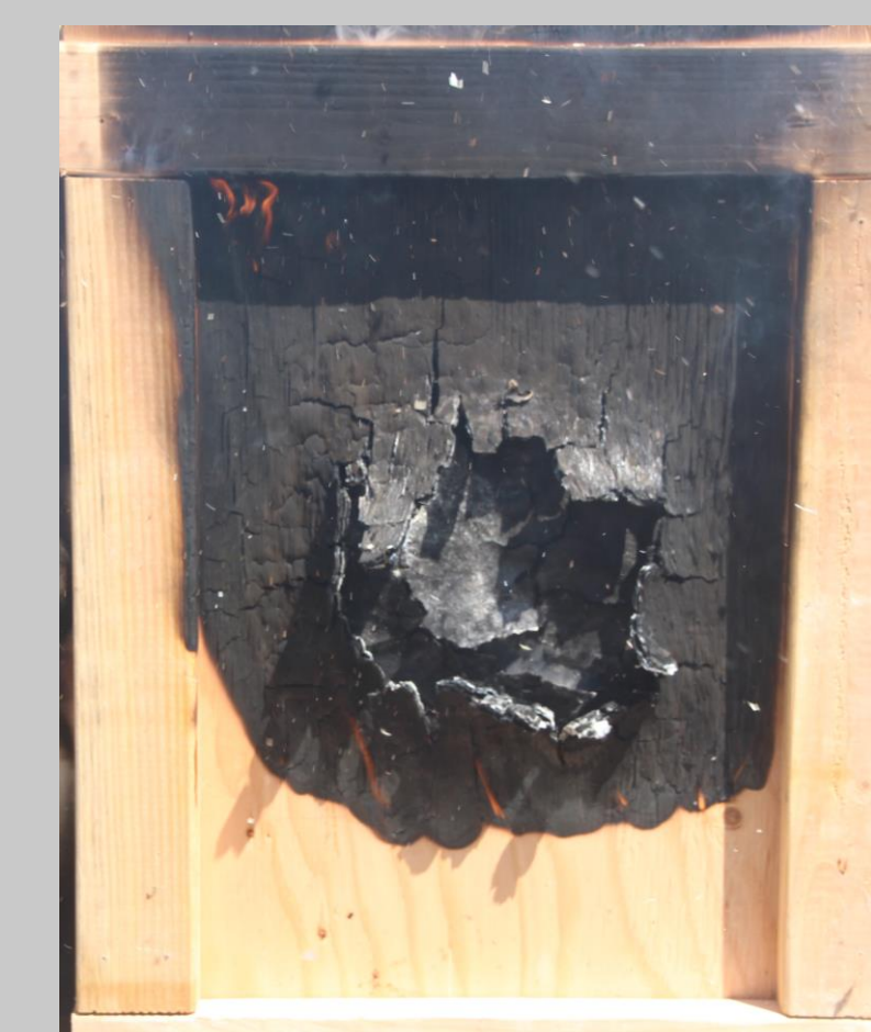
Figure 5: The back of the control roof after test completion
