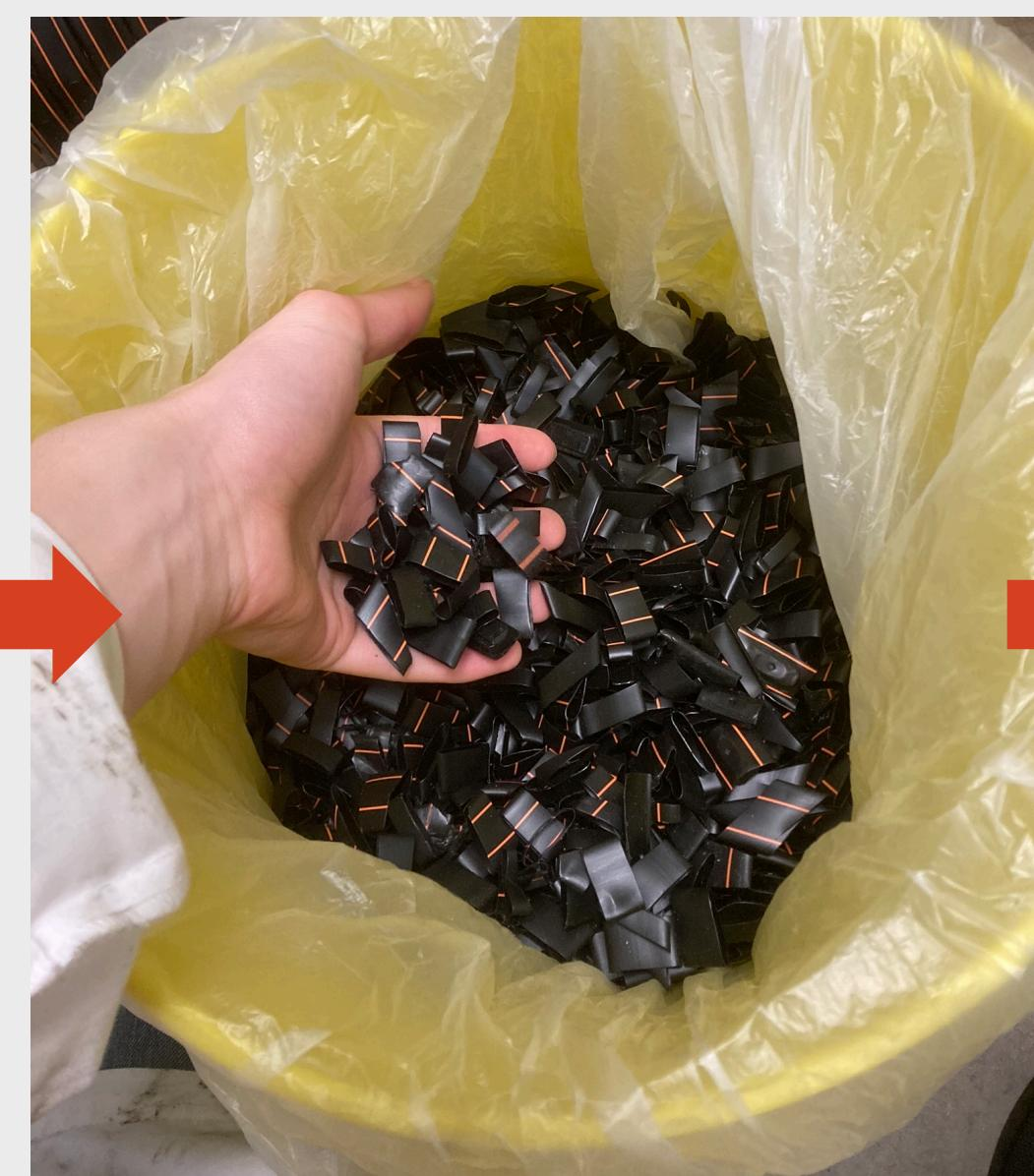
Plastic is cut down to size to be more easily compacted into the reactor
