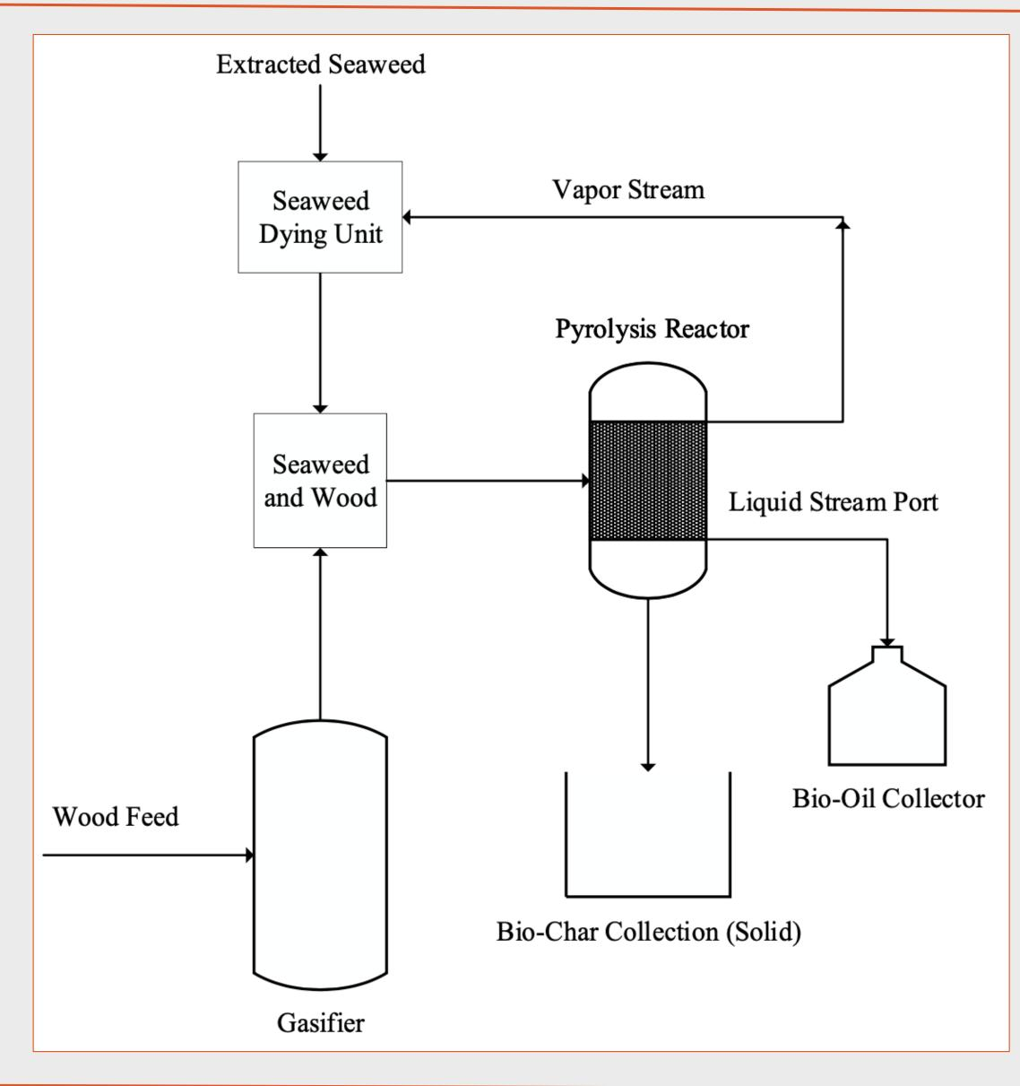
Process flow diagram for production of biochar and bio-oil from protein extraction residuals of Oregon Dulse seaweed and added forestry residuals (i.e. wood chips). A slow pyrolysis unit will be used to produce biochar while a gasifier burning wood chips will supply energy for the pyrolysis, as well as for the superheated steam dryer.
