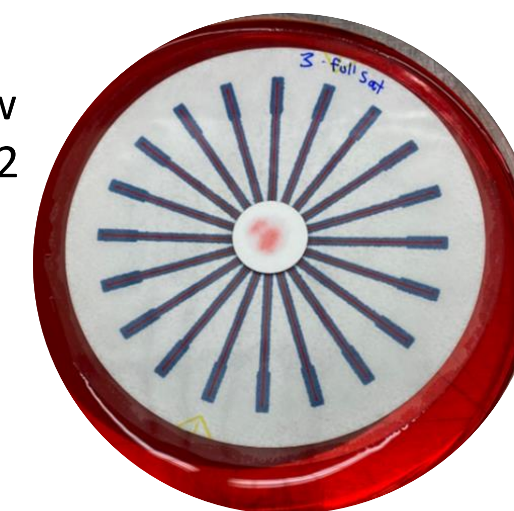
Hydrophobic wax printed channels
