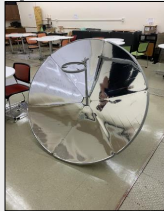
Figures: Our CAD model of the free piston Stirling engine (left). Parabolic solar cooker used for generating renewable heat to power the Stirling engine (right).
