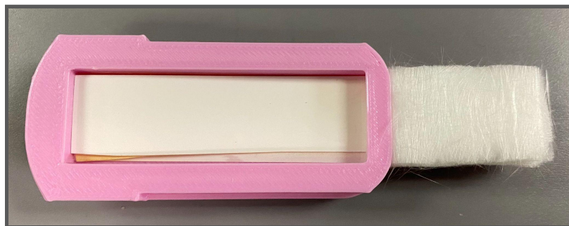
Figure VII. Final physical prototype with nitrocellulose strips and glass fiber sample pad
