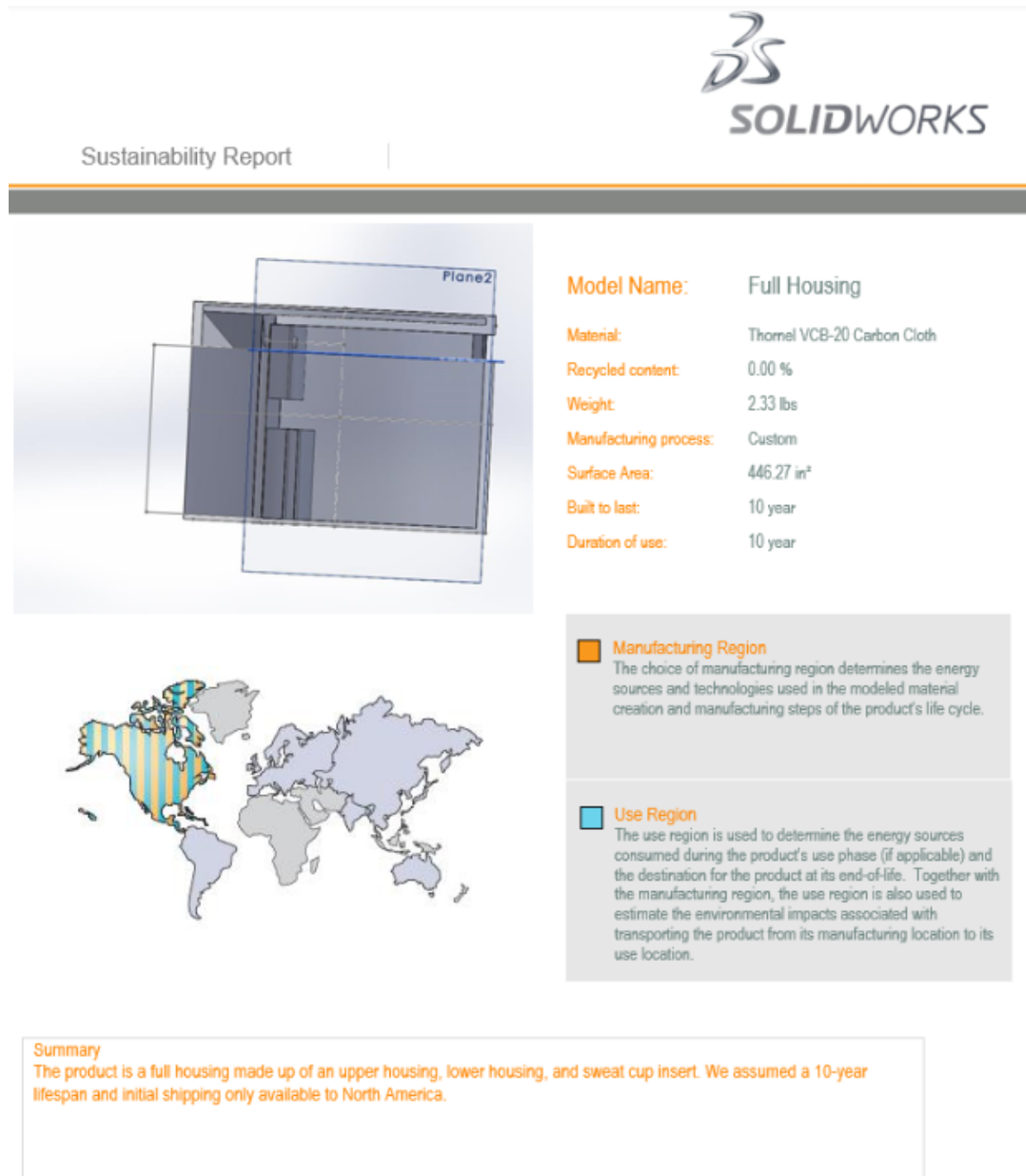
Figure 12 The sustainability report for the vacuum prosthetic socket design in the region will be manufactured and used.
