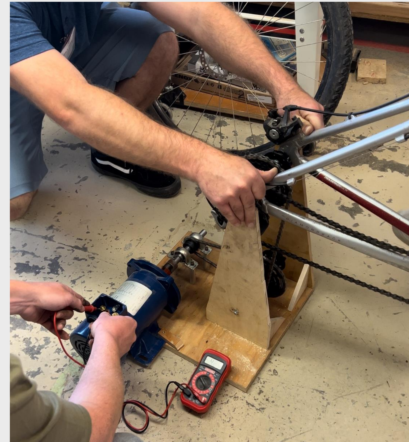
Figure 2: Team members testing voltage output of first prototype
