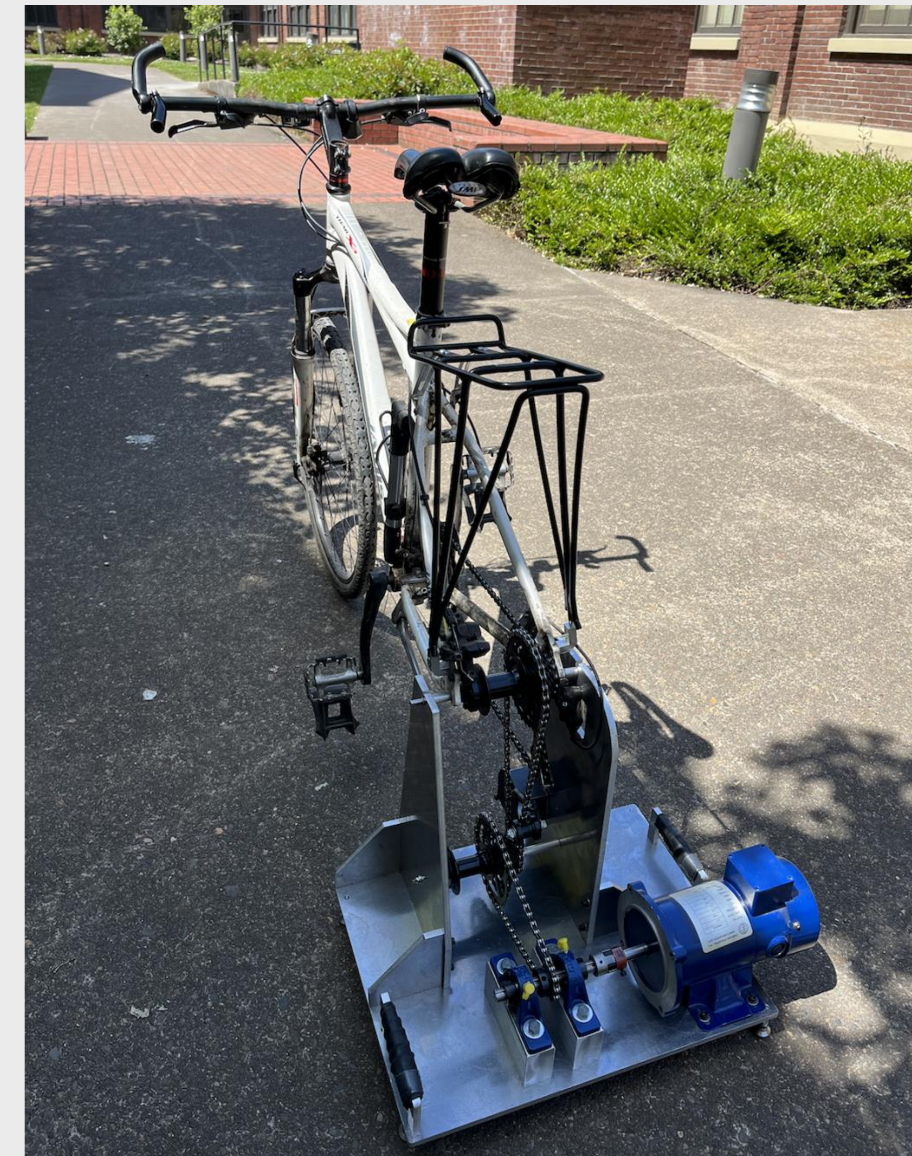
Figure 3: Completed final prototype w/ generator attachment
