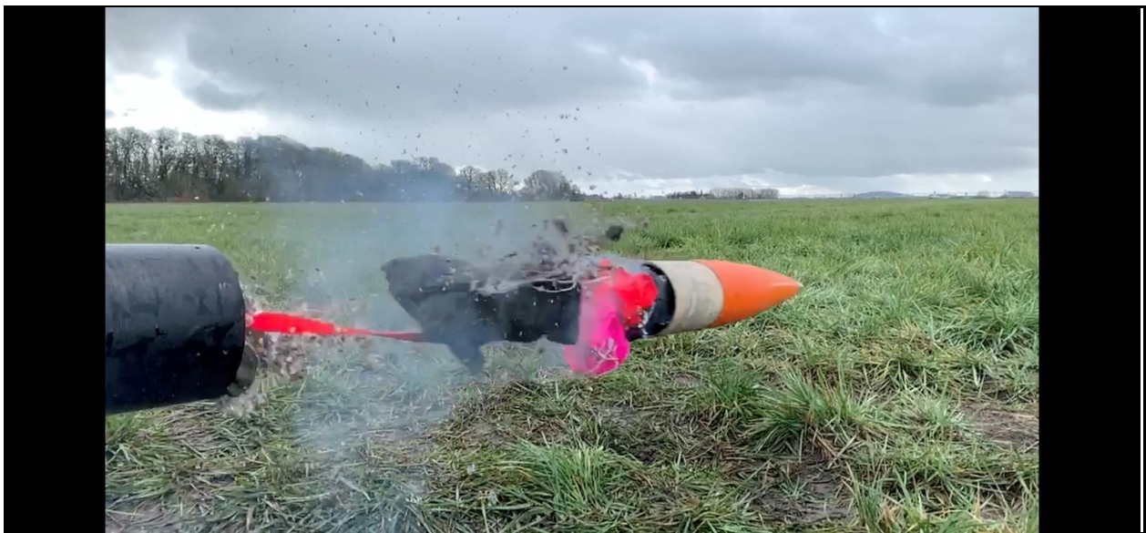
Figure 24. Successful main parachute ejection.
