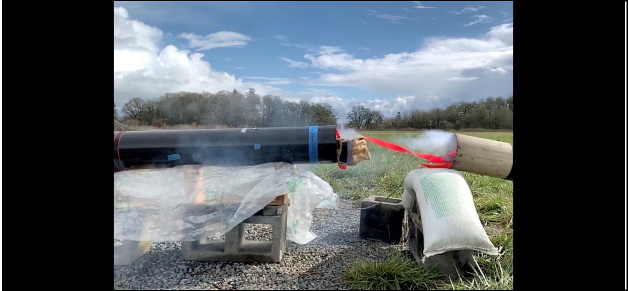
Figure 23. Successful drogue parachute ejection.
