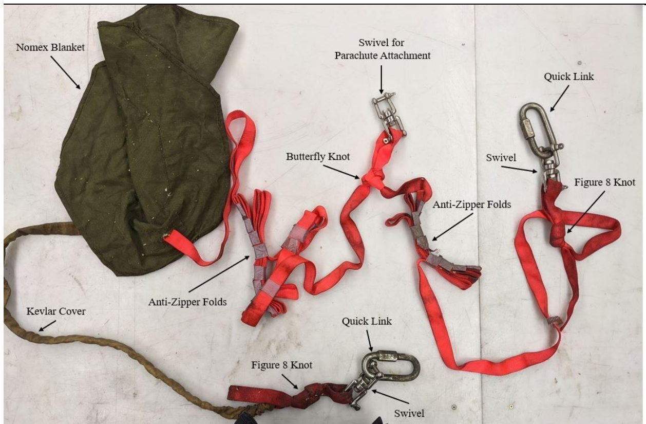
Figure 16. The drogue parachute recovery system components with labels.
