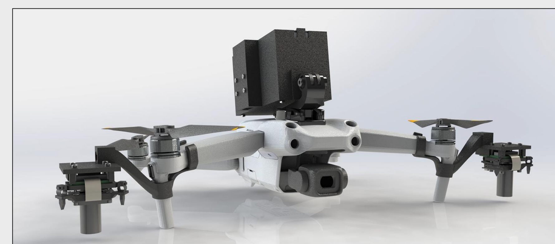
Figure 5. SVC final design with cameras mounted to the drone legs.
