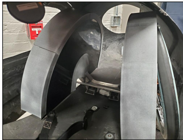
Figure 19. Final wheel shields in the vehicle.
