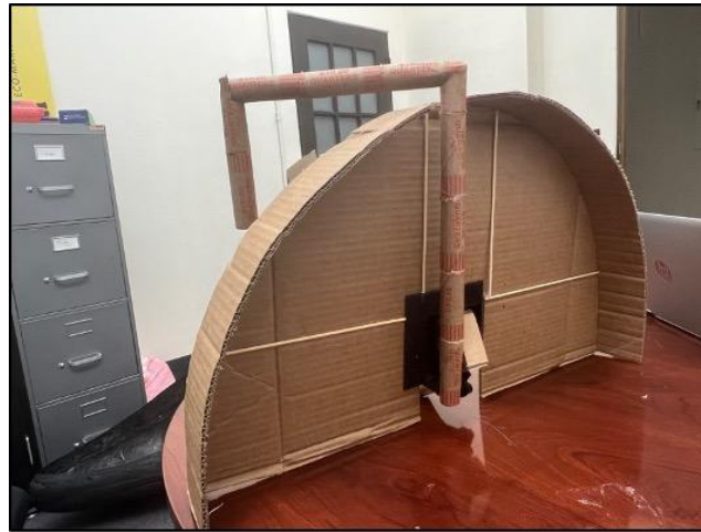
Figure 4. The proposed design solution for the tire shields, including the redesigned steering arm.
