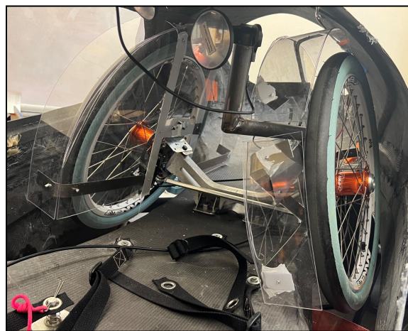
Figure 1. Original front axle assembly in OSU's Eco-Marathon vehicle.
