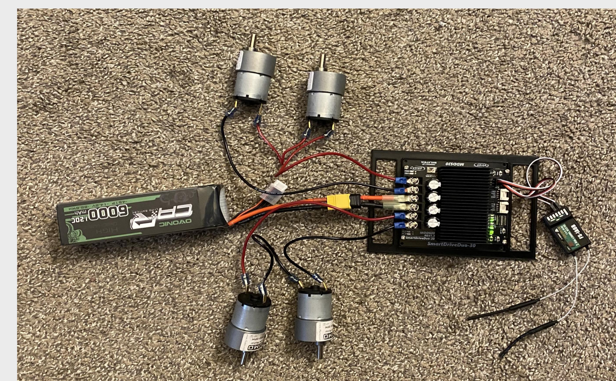
Figure 4. Fully Exposed Electrical Components
