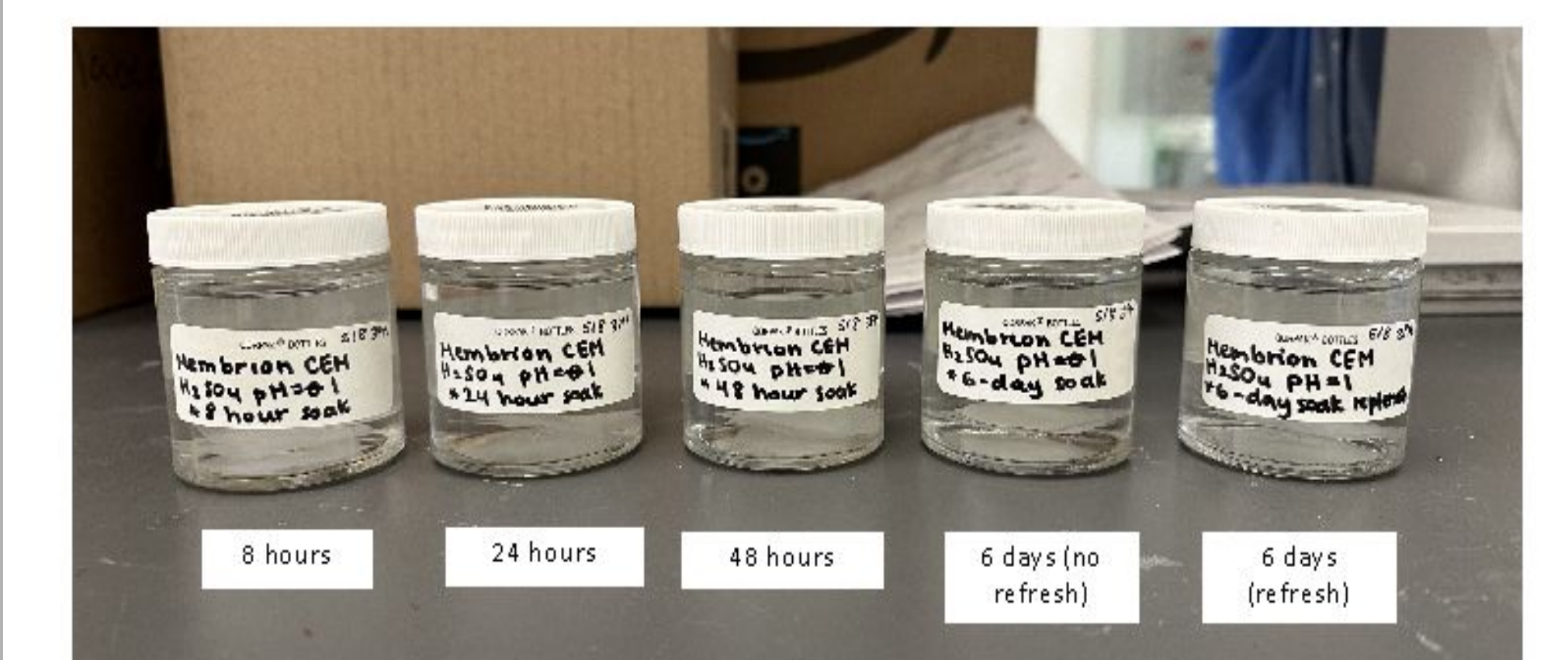
Figure 4. Membrane capacity testing conducted on long-term exposures of 6 days and 48 hours, and short-term exposures of 24 hours and 8 hours
