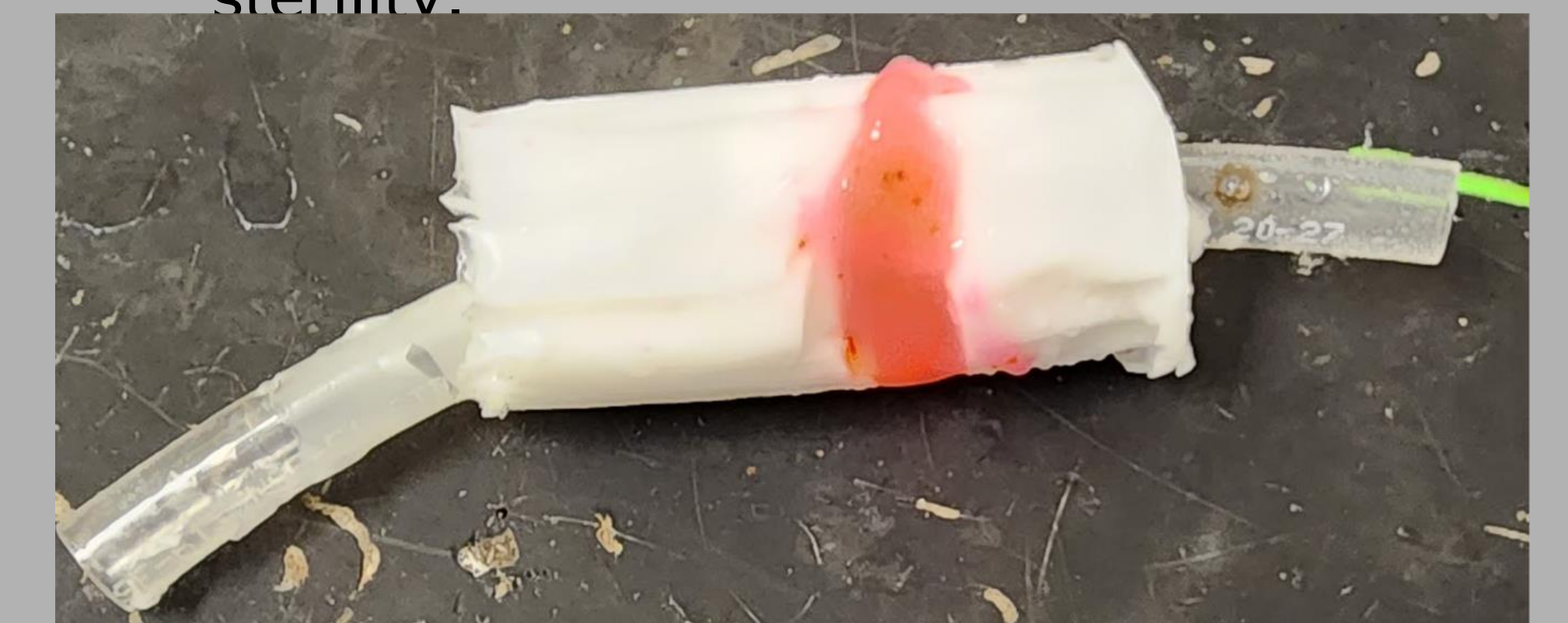
Figure 4. A rigid hydrogel was formed on the silicon test model when chitosan and genipin were sprayed from two different spray cans. Note that the hydrogel retains its form against gravity.
