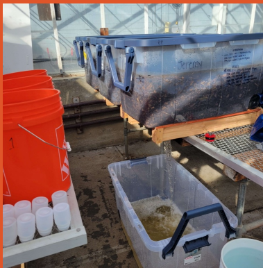
Figure 1: Experimental setup of three prototype woodchip bioreactors
