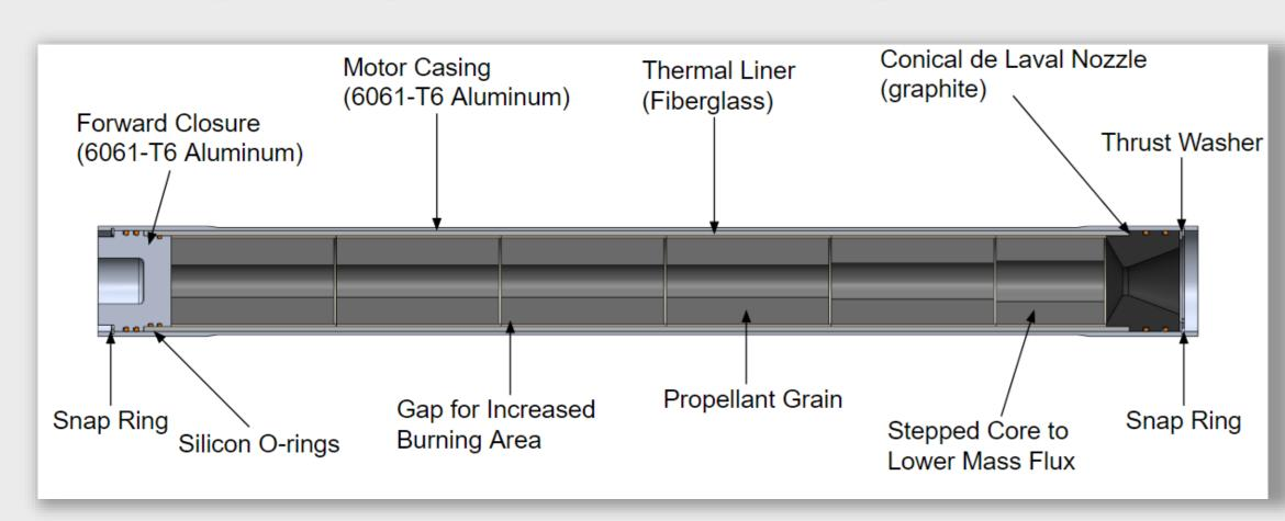
Snap rings are used to secure all motor components in place to increase the re-usability of the motor and decrease the severity of motor destruction in the event of a Catastrophic Take-off (CATO)
