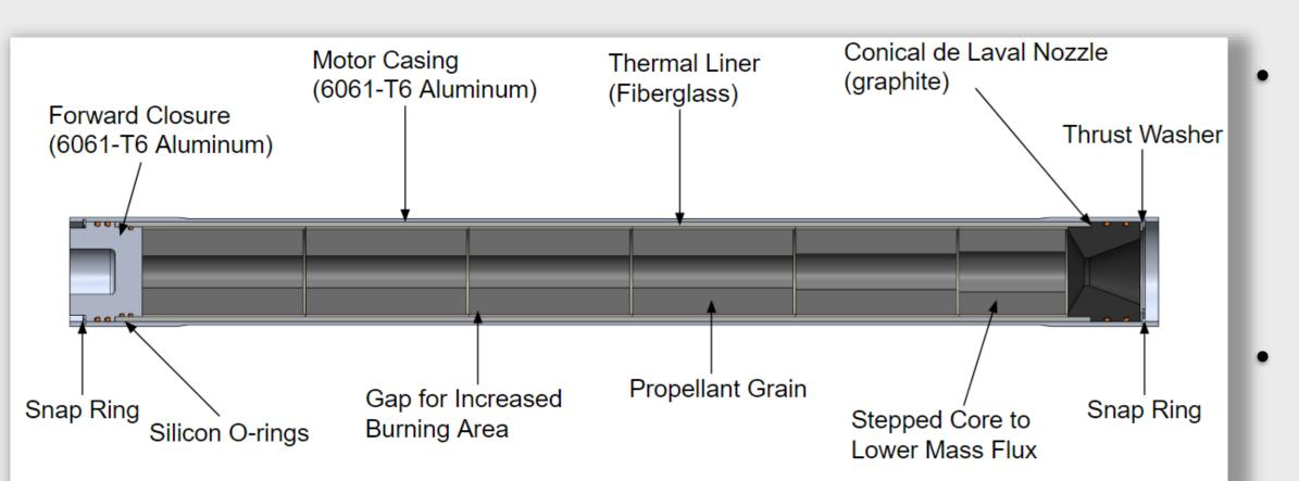
Snap rings are used to secure all motor components in place to increase the re-usability of the motor and decrease the severity of motor destruction in the event of a Catastrophic Take-off (CATO)
