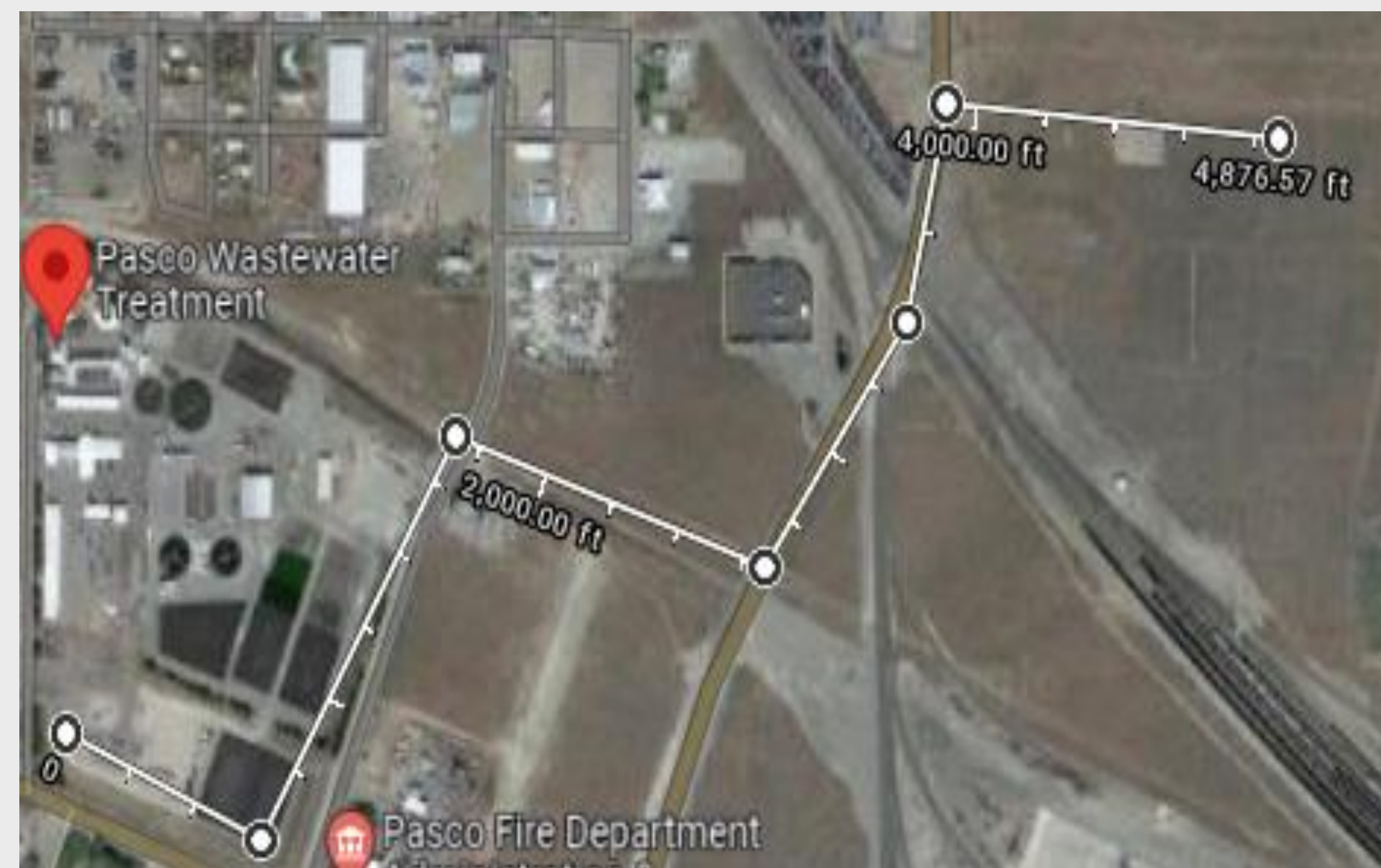
Proposed pipeline to pump reclaimed water from the local Wastewater Treatment facility to a holding tank.
