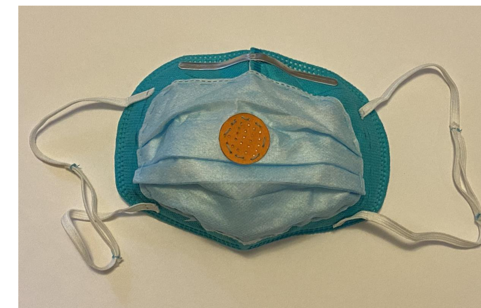
Figure 7: A physical prototype of our final design using N95 and surgical mask components, adjustable straps, and a paper substitute for the ruthenium complex.
