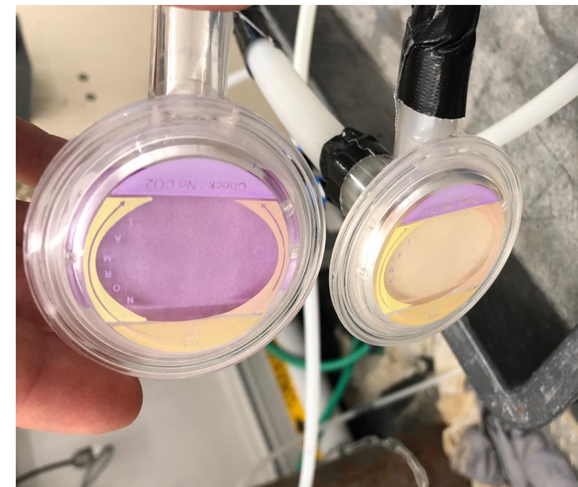
Figure 3: The Medline analogous carbon dioxide sensor used in modeling. The purple shows the base state, and the yellow represents increased concentration of carbon dioxide.
